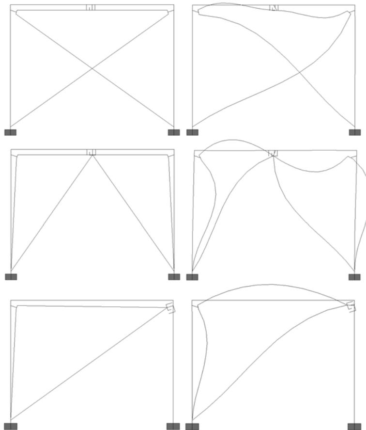
Figure 1 Static configuration and deformation of dual system 1, 2 and 3
