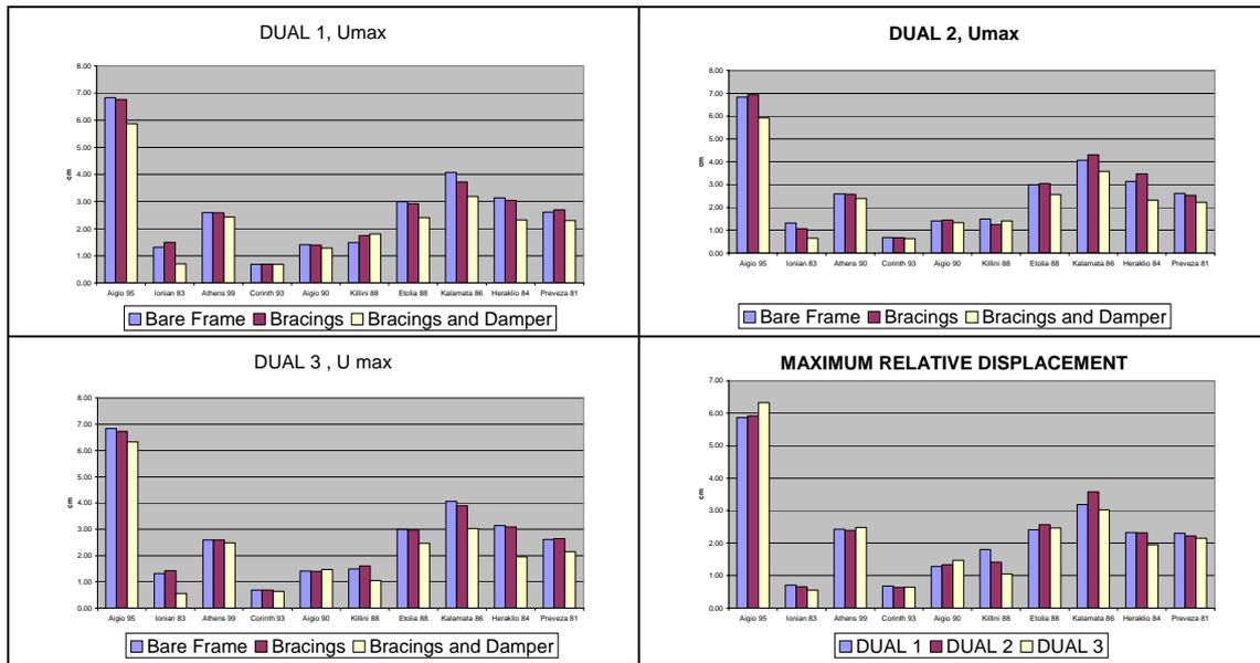
Figure 4 Relative displacements of dual systems
