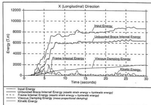
Figure 13: Seismic Energy Dissipation Plot
