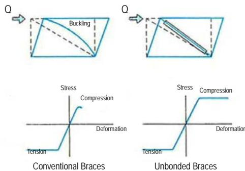
Figure 6: Conventional vs. Unbonded Braces
