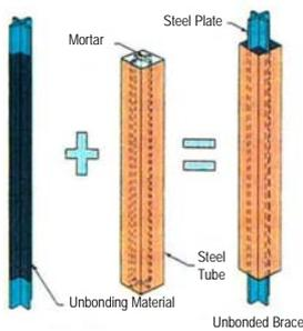
Figure 5: Unbonded Brace Diagram
