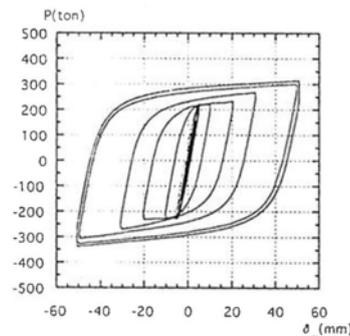
Figure 7: Unbonded Brace Hysteresis Curve
