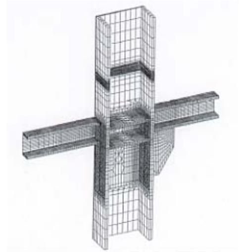
Figure 15: FEM Model of Column-Beam Joint
