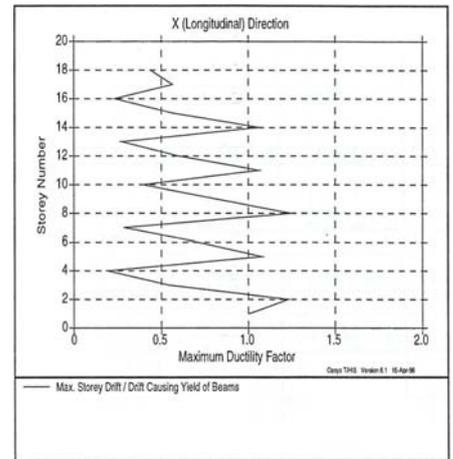
Figure 12: Ductility Factor of Main Structure
