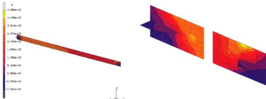
Figure 14: Unbonded Brace Analysis Result (elongation of 55 mm combined with self-weight)
