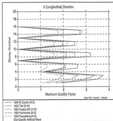
Figure 11: Ductility Factor of Unbonded Braces
