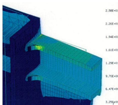
Figure 17: Column Beam Joint with round Haunch
