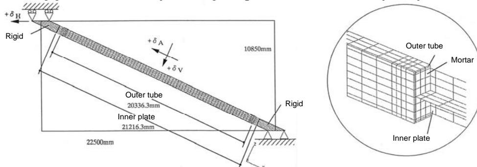
Figure 9: Unbonded Brace Analysis Model
