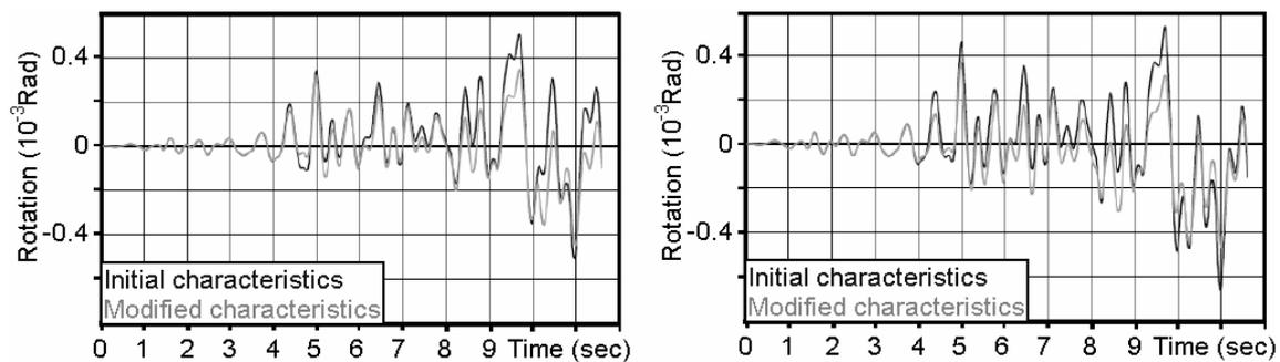
Figure 9. The rotations of the top of the bearing LRB1 of the end column Y8, for the earthquake of Thessaloniki, with a probability of exceedance of 10% in 50 years (left) and 10% in 100 years (right).
