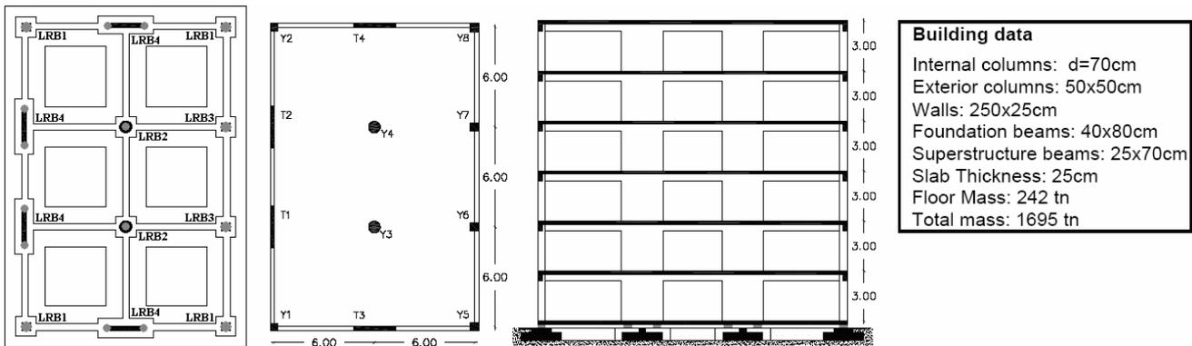
Figure 2 Plan view (foundation and superstructure) and elevation view of the building.
