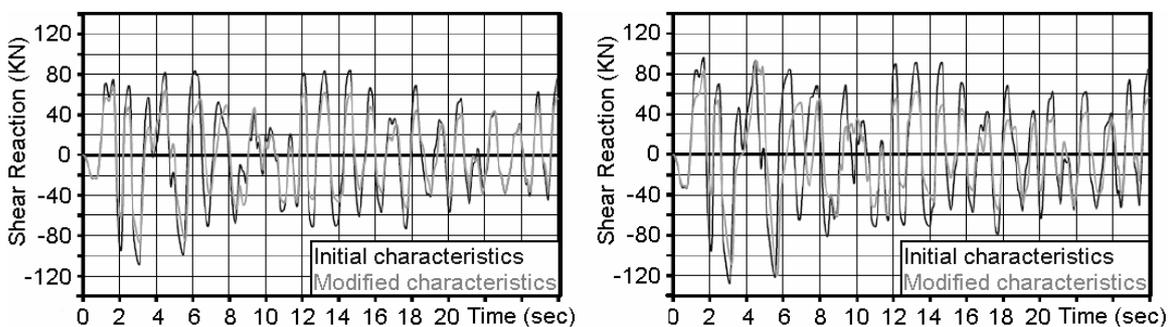
Figure 10. The shear force which develops in the bearing of the column Y4 for the earthquake of El Centro with a probability of exceedance of 10% in 50 years (left) and 10% in 100 years (right).
