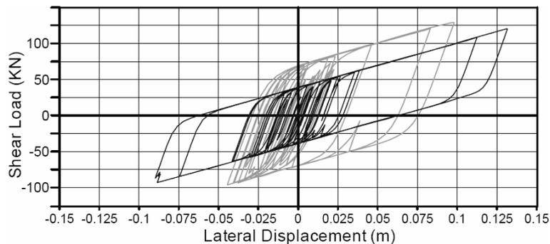
Figure 7 The hysteresis loops of LRB2 bearing for the El Centro earthquake with probability of exceedance of 10% in 100 years, before (gray) and after (black) the characteristics' change due to temperature rises.
