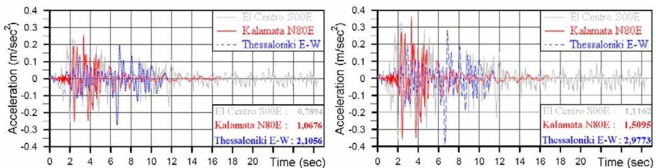
Figure 3 Scaled earthquakes motions with exceedance probability: 10% in 50 years (left) and 100 years (right).
