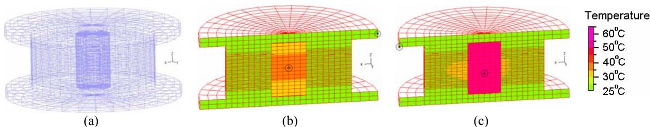
Figure 1 The form of the micromodel which has been used for the thermo mechanical analysis (a) and (b, c) the change of the temperature in various time steps of the analysis.
