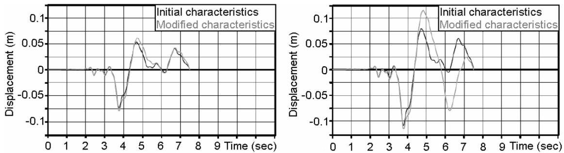
Figure 8. The displacement of the diaphragm over the seismic isolation system for the earthquake of Kalamata with a probability of exceedance of 10% in 50 years (left) and 10% in 100 years (right).
