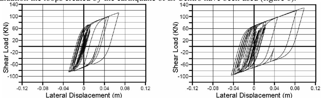
Figure 6 The hysteresis loops of LRB2 bearing for the El Centro earthquake with probability of exceedance of 10% in 50 years (left) and 10% in 100 years (right).
