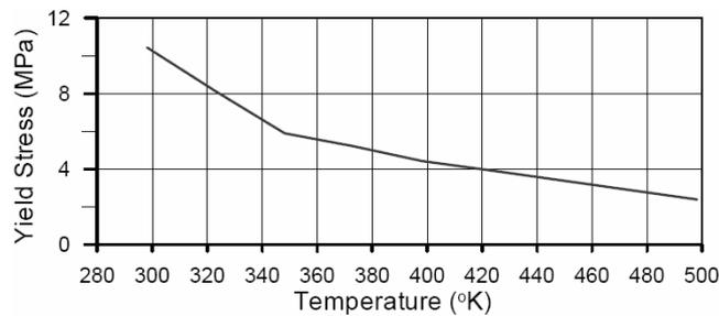
Figure 5 The change of stress leakage of the lead core for different temperatures.
