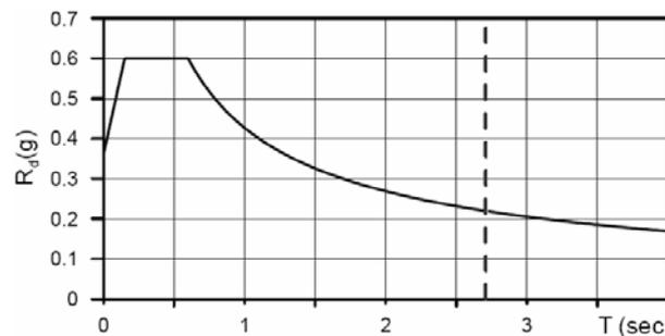
Figure 4 Spectrum acceleration according to Greek Seismic Code, for  $A=0,36g$  and  $q=1.5$ .
