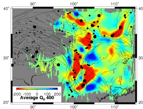
Fig.3 Imaged  $Q_0$  lateral variations and large earthquakes distribution
