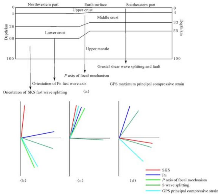
Fig.6 Physical parameters manifesting stress-strain orientation of each layer in Yunnan and its adjacent areas and zoning distribution of average orientation of each layer
