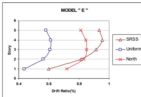
Fig. 8. Drift of the storey in structure (E) under different loading conditions
