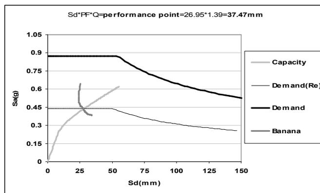
Fig. 5. Determination of performance point for structures A in (SRSS) load pattern
