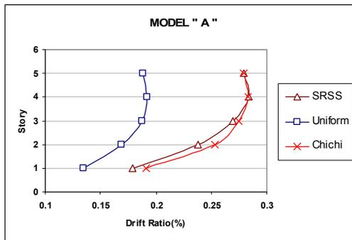
Fig. 6. Drift of the storey in structure (A) under different loading conditions
