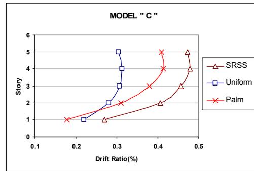
Fig. 7. Drift of the storey in structure (C) under different loading conditions
