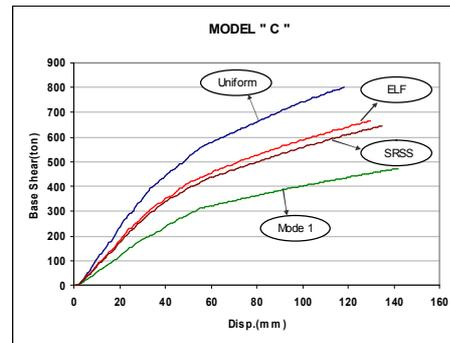
Fig. 3. Capacity curve for structure C under different loading conditions
