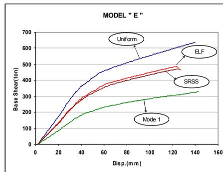
Fig. 4. Capacity curve for structure E under different loading conditions
