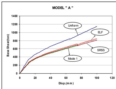
Fig. 2. Capacity curve for structure A under different loading conditions
