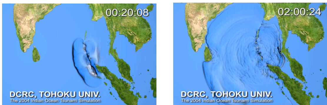
Figure 1 Snapshot of the tsunami propagation at 20 minutes and 2 hours after the generation. The first motion of the tsunami was positive in Sri Lanka and negative in Thailand
