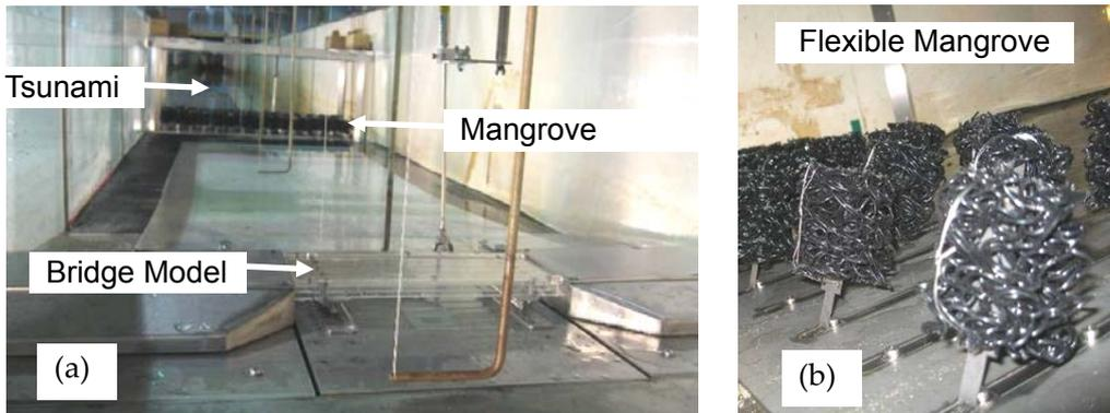
Figure 2 Photograph of mangrove models (a) position (b) flexible trunks
