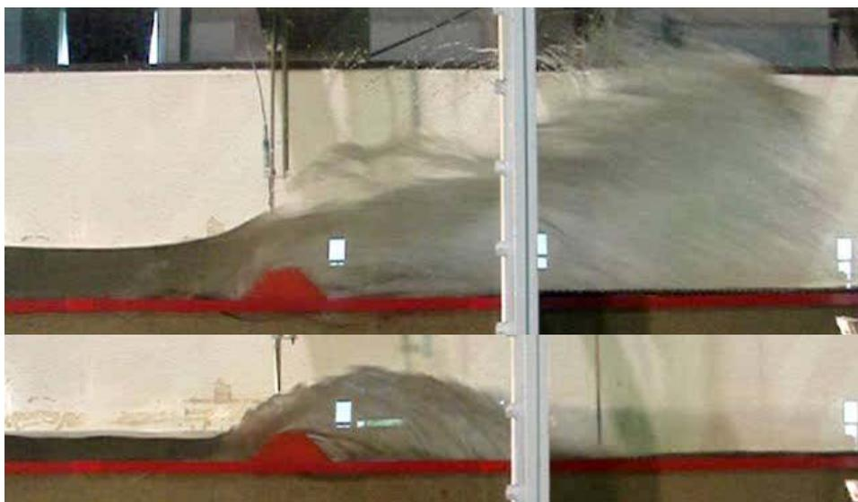
Figure 11 Photograph of tsunami hitting breakwater (a) high level tsunami (b) low level tsunami
