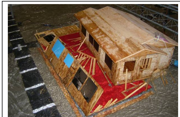
Figure 6. 1/6 th scale residential structure that was tested to failure by wave impact.
