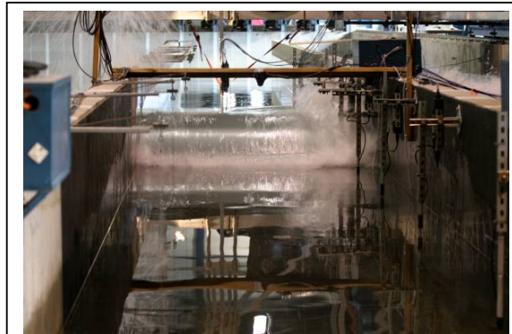
Figure 5. A solitary breaking wave in one of two flume channels instrumented to measure runup.
