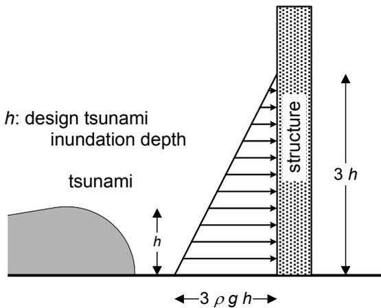
Figure 2 Design tsunami pressure distribution (JCO 2005)
