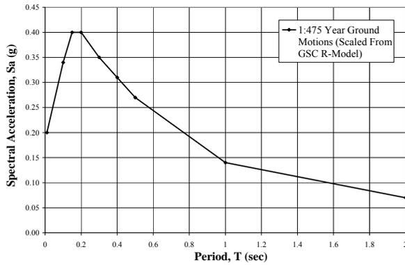
Figure 8: Uniform Hazard Response Spectrum
