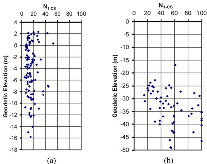
Figure 5: Interpreted Penetration Resistance Profiles
