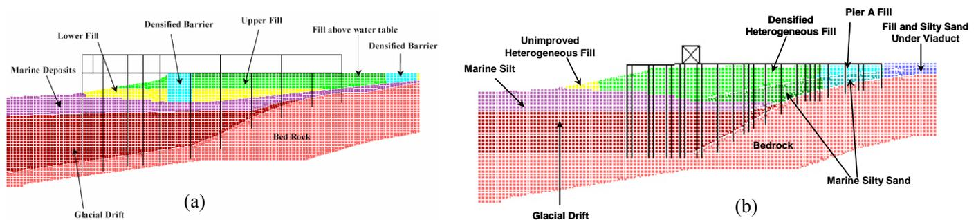
Figure 8: FLAC Finite Difference Models Used to Discretize the Drilled Shaft and Pile Foundation Schemes
