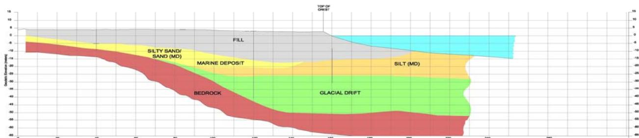
Figure 4: Typical Soil Stratigraphy Along A North-South Section (Looking West)
