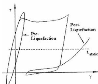
Figure 7a: Idealized Stress-Strain Behaviour
