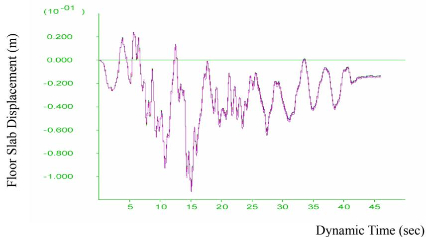
Figure 10: Horizontal Displacement Time-Histories of Floor Slab (475-yr Loading)
