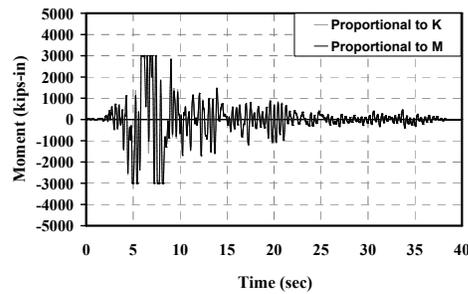
Figure 4: (a) Column end moments of Model A, (b) column end moments of Model B
