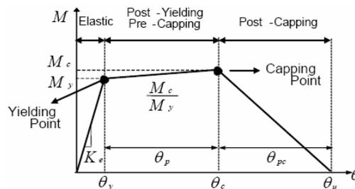
Figure 6: Structural component back bone curve
