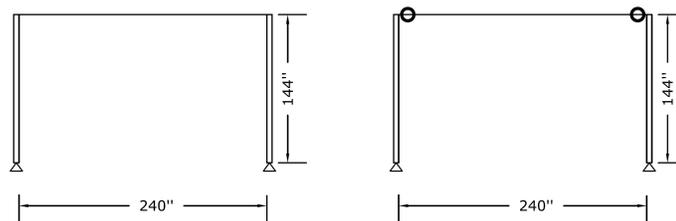
Figure 2: (a) Model without rotational springs, (b) Proposed model with rotational springs
