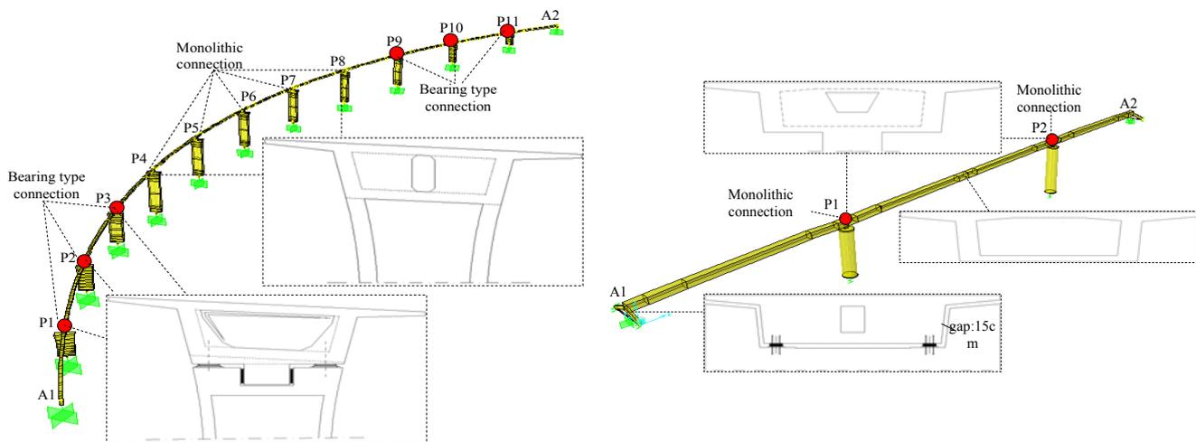
Figure 1 Layout of the Krystallopigi bridge and overcross bridge finite element modelling
