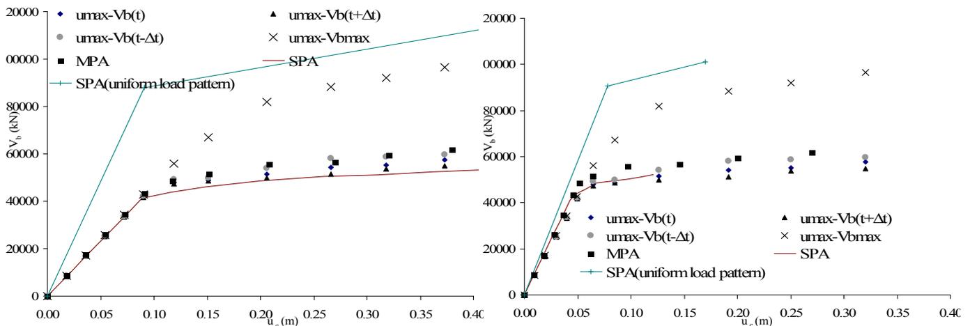
Figure 4 Pushover curves derived from SPA(first mode), SPA(uniform load), improved MPA and RHA for Krystallogipi bridge, derived with respect to the max deck displacement (deck mass centre) (left) and the deck displacement over P4
