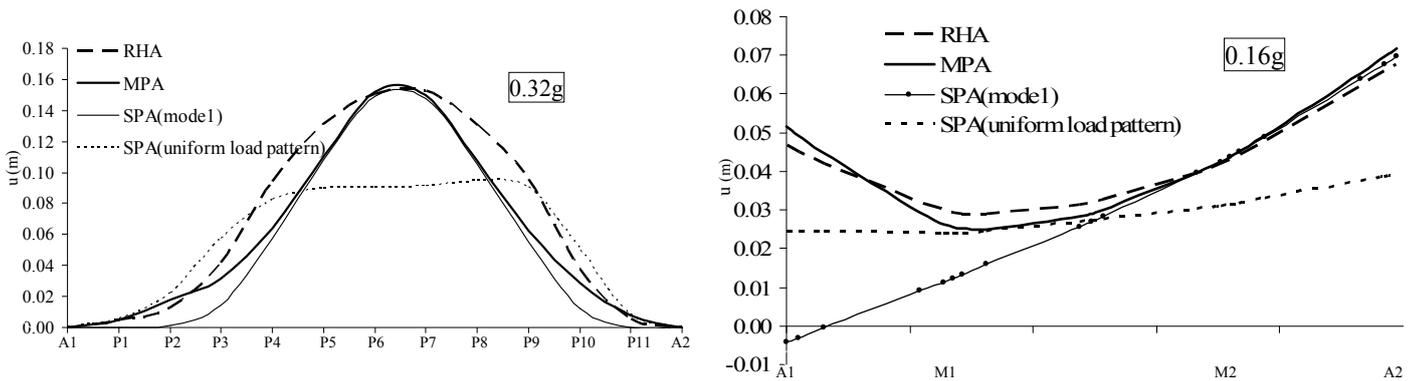
Figure 3 Response to the design earthquake calculated from SPA, MPA and RHA: deck displacements of the Krystallogipi bridge (left) and the overcross bridge (right).
