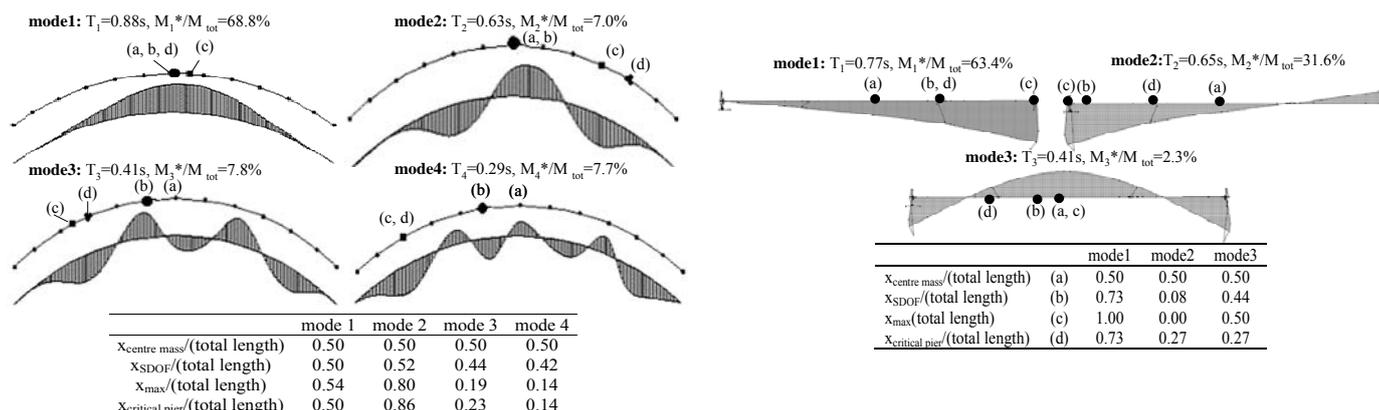
Figure 2 Modal force distribution, location of the equivalent SDOF systems and modal parameters for the main transverse modes of the Krystallopiigi bridge (left) and the overcross bridge.
