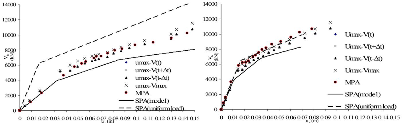
Figure 5. Pushover curves derived from SPA(first mode), SPA(uniform load), improved MPA and RHA for the overcross bridge, derived with respect to the maximum deck displacement (point A2) (left) and the deck mass centre.
