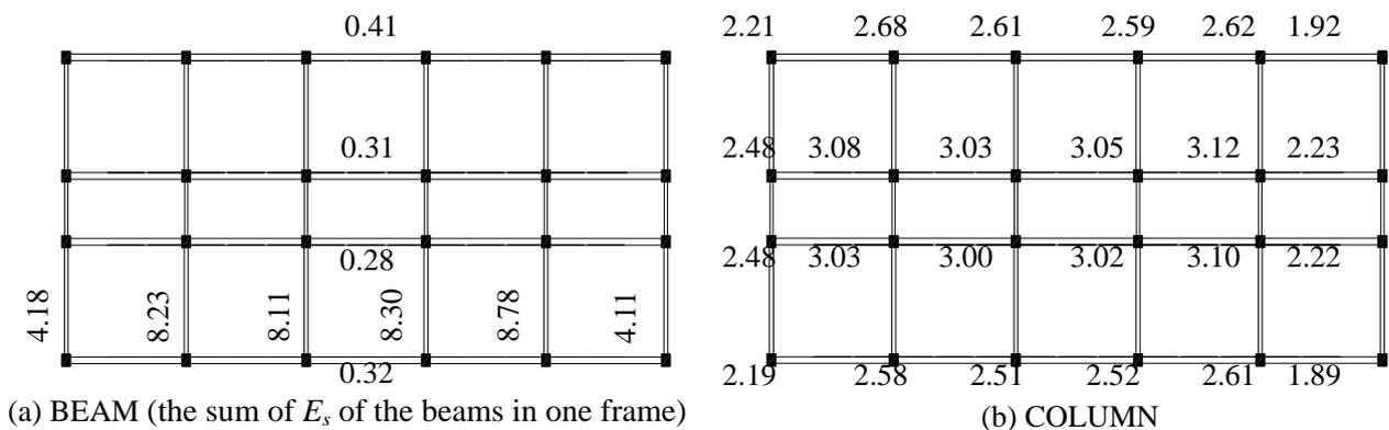
Figure 5. Detailed  $E_s$  distribution in first story (unit: kN·m)
