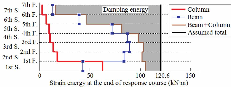
Figure 3. Disassembled strain energy distribution
