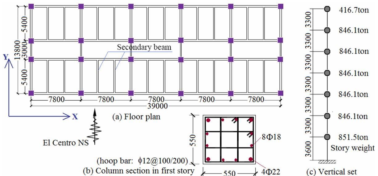
Figure 1. Scheme of the building model (dimension in mm)
