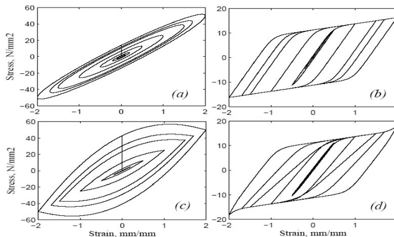
Figure 3. Examples of EDD's behaviors. (a): Maxwell model. (b): Bilinear inviscid plastic model. (c): Non linear dashpot. (d): Rubber model.
