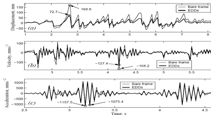
Fig. 6. Time history responses. (a): Horizontal displacement. (b): Velocity. (c): Acceleration.
