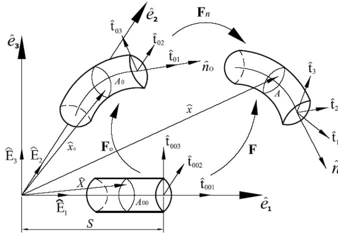
Figure 1. Configurational description of the beam.
