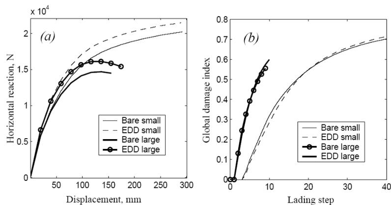
Figure 5. (a): Capacity curves. (b): Evolution of the global damage index.
