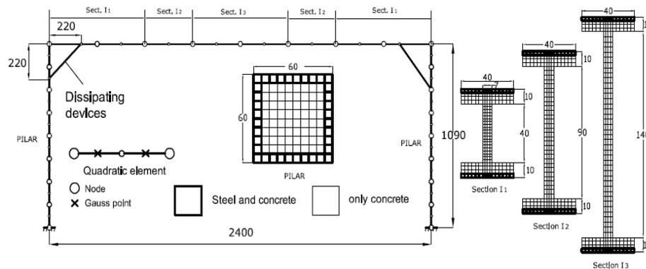
Fig. 4. Numerical model of the precast frame with energy EDDs and cross sectional meshes.
