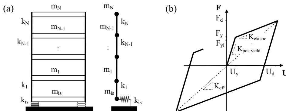
Figure 1: (a) Model of an N-story seismically isolated structure, (b) bilinear hysteretic model of the isolator.
