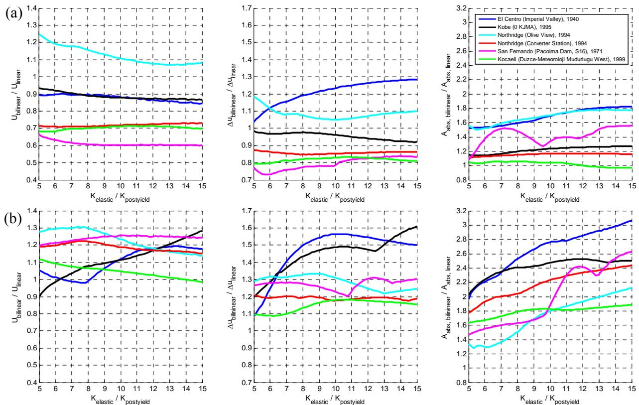
Figure 3: Ratio of the equivalent linear elastic analyses results to those of the bilinear inelastic analyses for varying ratio  $K_{elastic}/K_{postyield}$  under  $PGA = 0.5$  g: (a) 3-story and (b) 5-story building.
