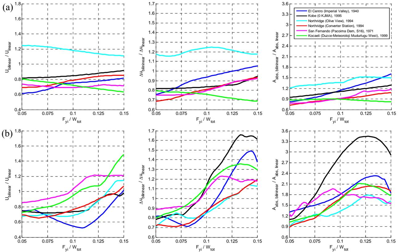
Figure 6: Ratio of the equivalent linear elastic analyses results to those of the bilinear inelastic analyses for varying ratio  $F_{yi}/W_{\text{tot}}$  under  $PGA = 1.0 \text{ g}$ : (a) 3-story and (b) 5-story building.
