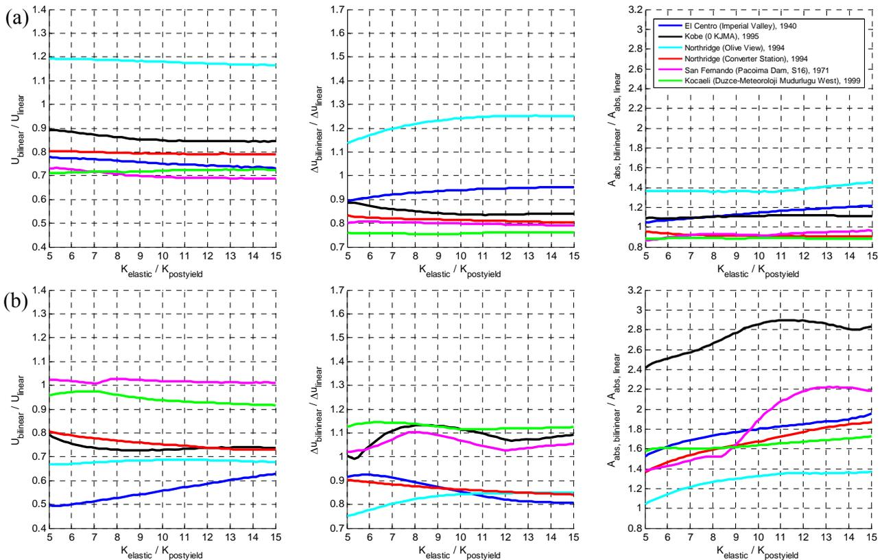
Figure 4: Ratio of the equivalent linear elastic analyses results to those of the bilinear inelastic analyses for varying ratio  $K_{elastic}/K_{postyield}$  under  $PGA = 1.0\text{ g}$ : (a) 3-story and (b) 5-story building.
