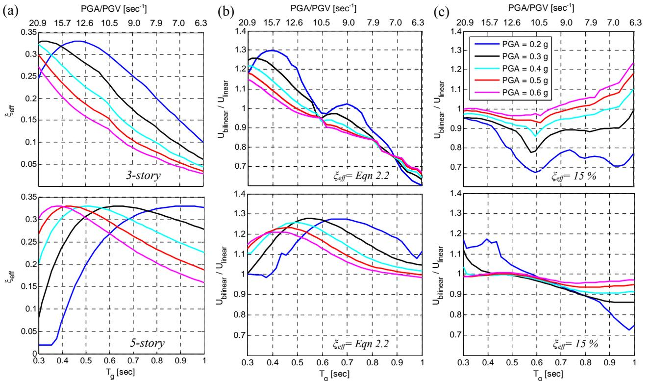
Figure 2: (a) Effective damping according to Eqn 2.2, (b, c) Maximum isolation displacement ratio with  $\zeta_{eff}$  calculated from Eqn 2.2 or set to a constant 15 % value, respectively.
