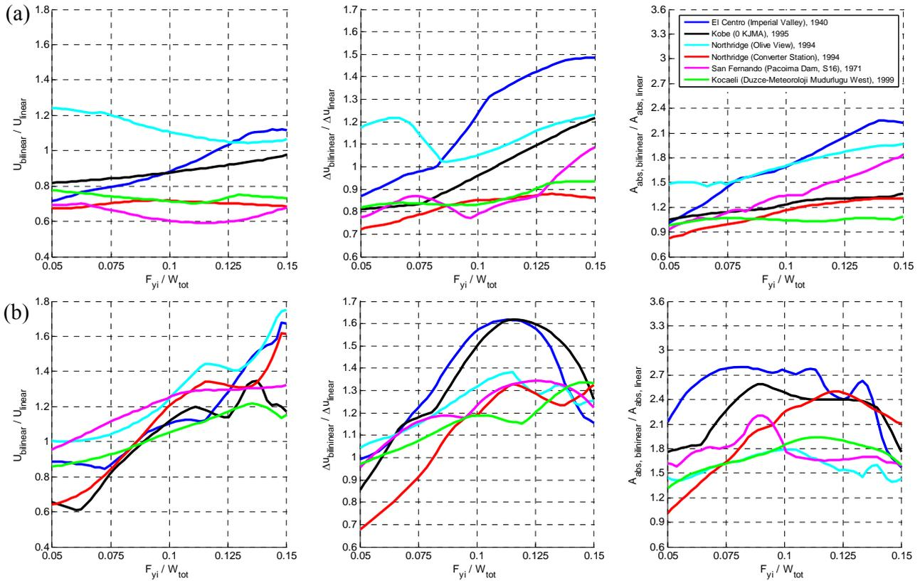
Figure 5: Ratio of the equivalent linear elastic analyses results to those of the bilinear inelastic analyses for varying ratio  $F_{yi}/W_{\text{tot}}$  under  $PGA = 0.5 \text{ g}$ : (a) 3-story and (b) 5-story building.
