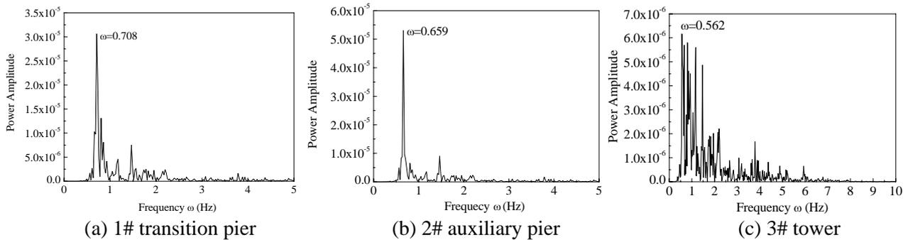
Figure 9 FFT results of the pile caps' acceleration response under longitudinal seismic excitation
