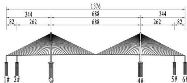
Figure 1 Layout of the bridge (Unit: m)
