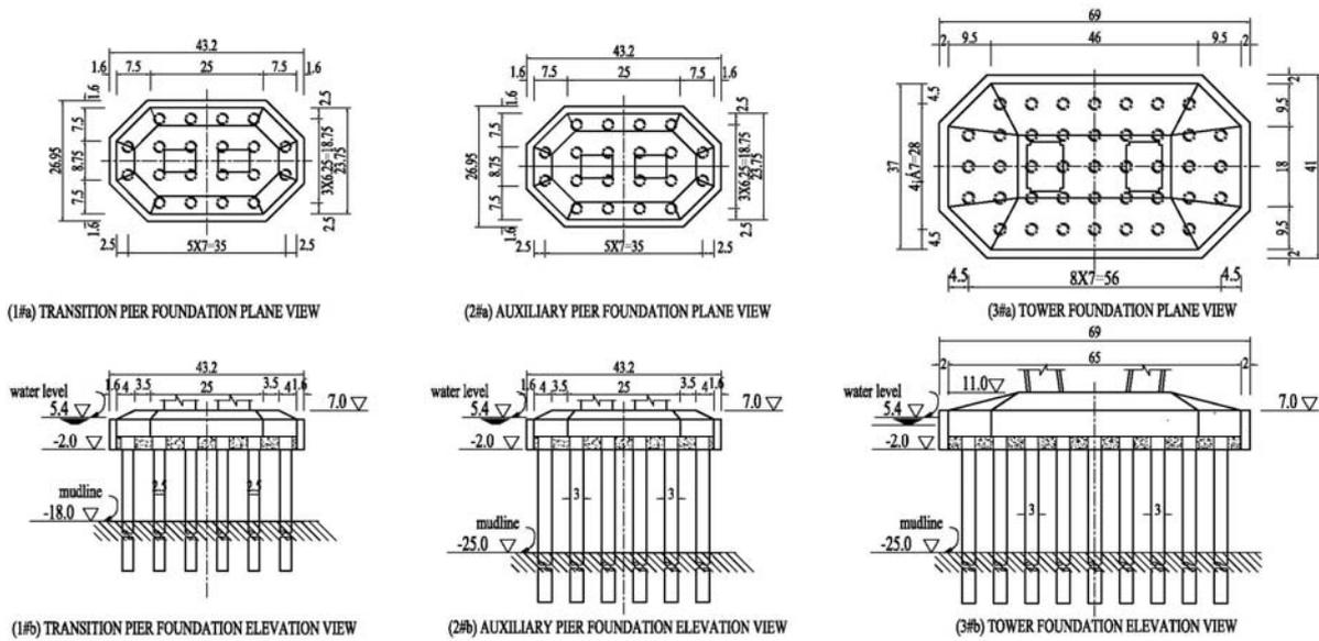
Figure 5 Pile foundations' geometry of the bridge (Unit: m)
