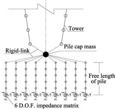
Figure 2 Individual pile model
