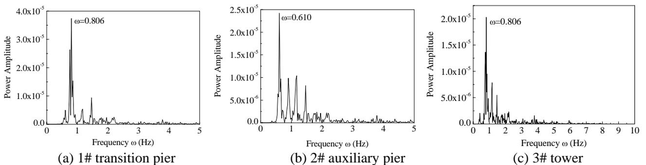
Figure 10 FFT results of the pile caps' acceleration response under transverse seismic excitation
