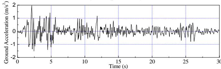
Figure 8 El Centro N-S earthquake wave records with scaled PGA of 0.2g
