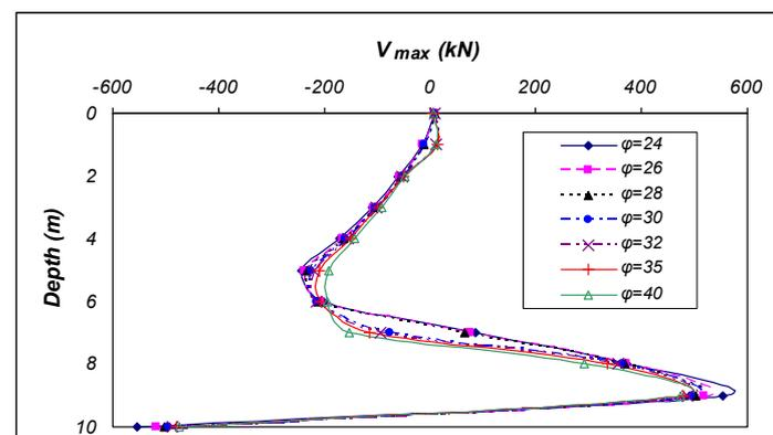
Figure 8 Maximum shear forces in the pile versus sand friction angle
