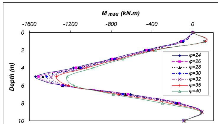
Figure 9 Maximum bending moments in the pile versus sand friction angle
