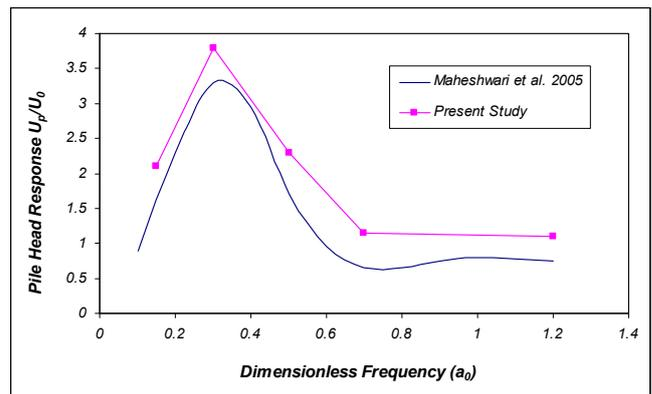
Figure 3 Dynamic verification for pile-head response
