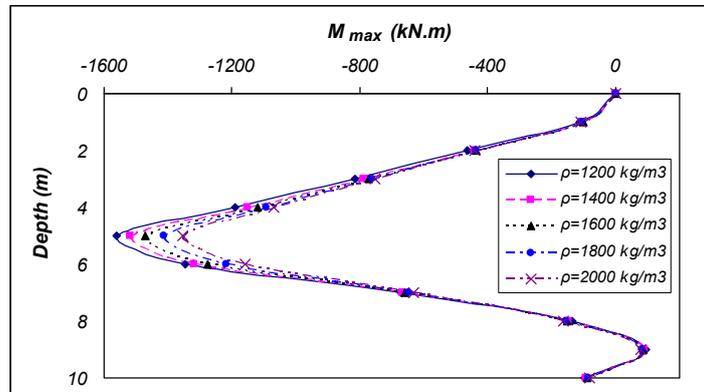
Figure 6 Maximum bending moments in the pile versus sand density
