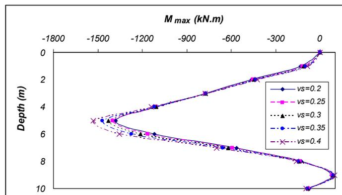
Figure 13 Maximum bending moments in the pile versus sand Poisson's ratios
