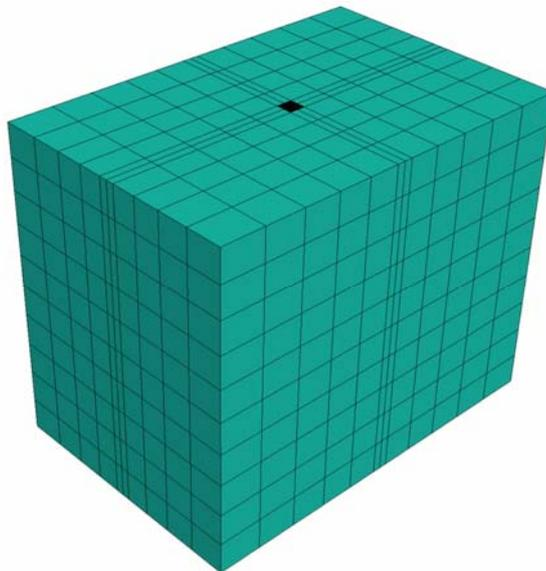
Figure 1 Three-dimensional finite element model used for the soil-pile system
