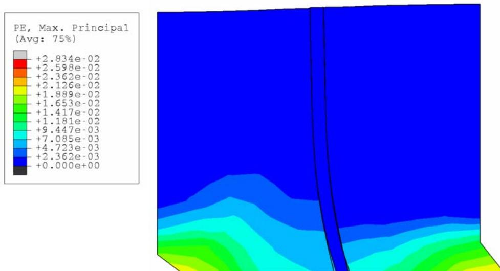
Figure 10 Plastic strains near the pile ( $\phi= 40^\circ$ )
