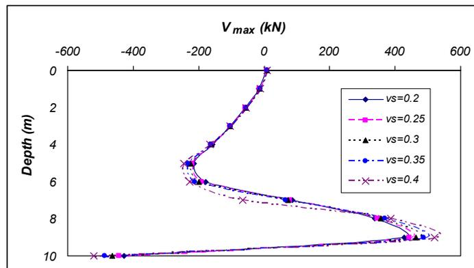
Figure 12 Maximum shear forces in the pile versus sand Poisson's ratios
