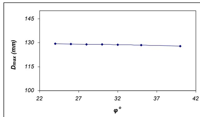
Figure 7 Maximum pile deflections versus sand friction angle
