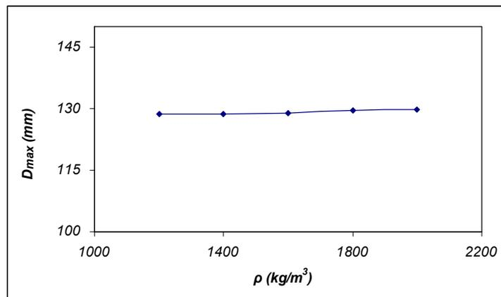
Figure 4 Maximum pile deflections versus sand density
