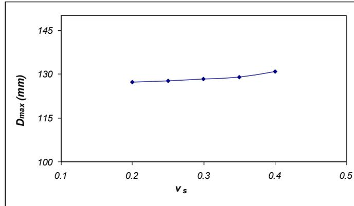
Figure 11 Maximum pile deflections versus sand Poisson's ratios
