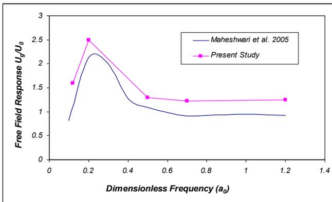
Figure 2 Dynamic verification for free-field response
