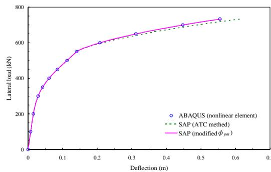
Figure 8 Capacity curves for free-head condition
