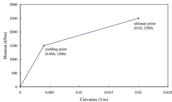
Figure 5 Moment-curvature curves of the pile
