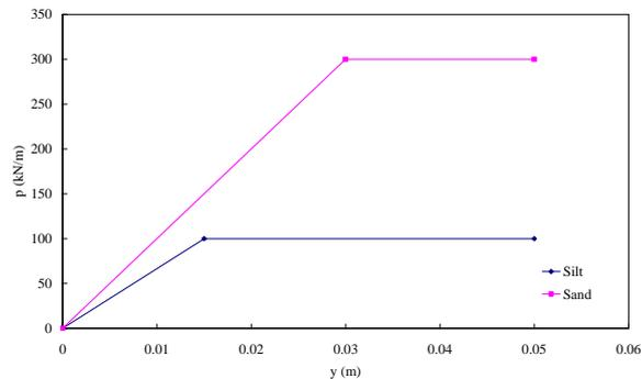
Figure 6  $p$ - $y$  curves of soil layers
