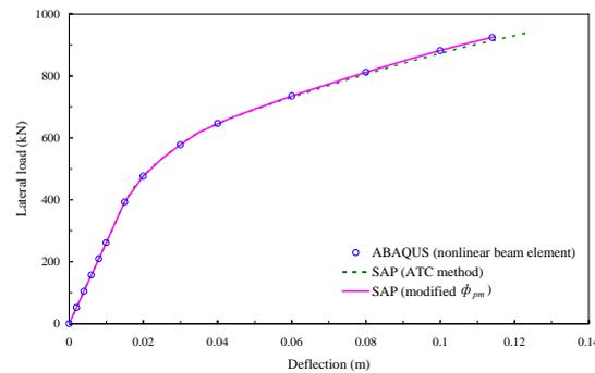
Figure 9 Capacity curves for fixed-head condition
