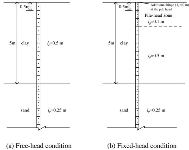
Figure 7 Arrangement of distributed plastic hinges in SAP analysis
