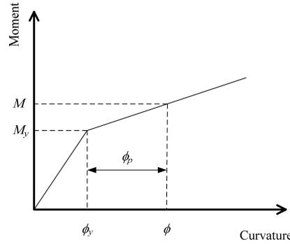
Figure 1 Plastic curvature defined in ATC-40 (1996)
