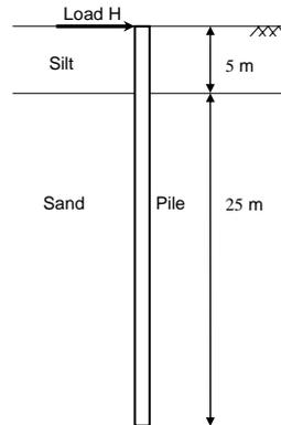
Figure 4 Example problem of a laterally loaded pile
