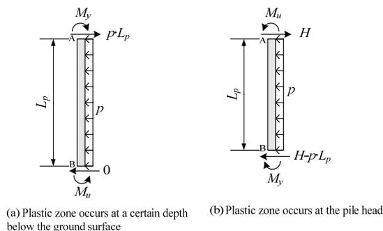
Figure 3 Free-body diagrams of plastic zones
