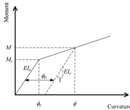
Figure 2 Modification for definition of plastic curvature
