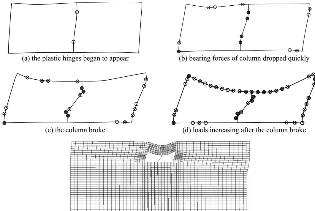
(e) the deformation of the soil-structure system corresponding to figure (d)
