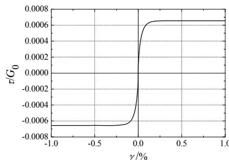
Fig. 4 Elasto-plastic stress- strain skeleton curve
