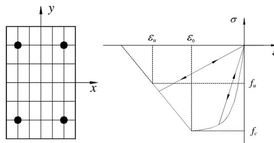
Fig. 3 Fiber model of reinforced concrete members and material constitutive model of concrete
