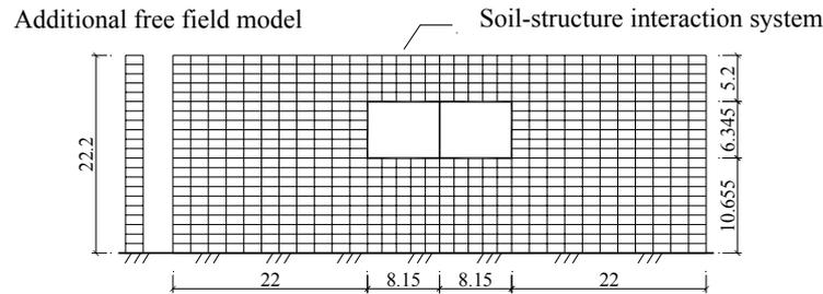
Fig. 2 Finite element model of soil-structure interaction system with additional free field (unit: m)
