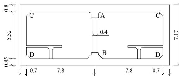
Fig. 1 Typical cross section of Daikai subway station (unit: m)
