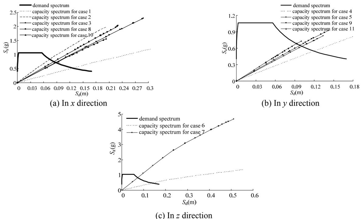
Fig.6 Determination of performance point for the stadium
