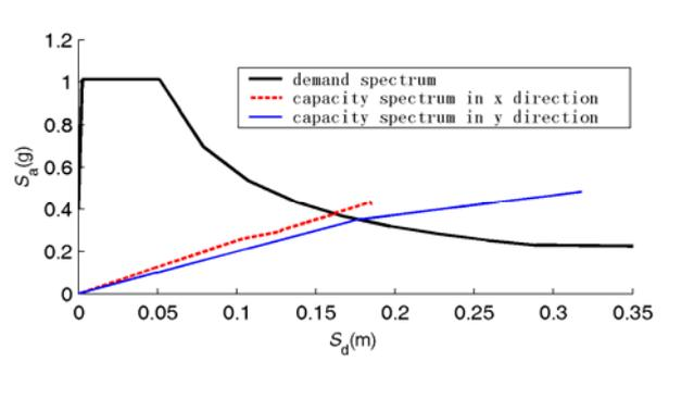
Fig.4 Determination of performance point for A380 hanger
