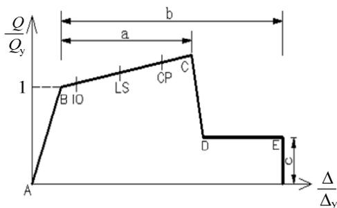
Fig.2 Generalized force-generalized displacement relationship curve of plastic hinges
