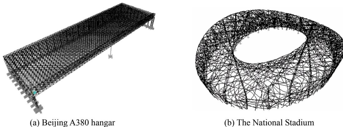
Fig.1 Analytical model of the two structures
