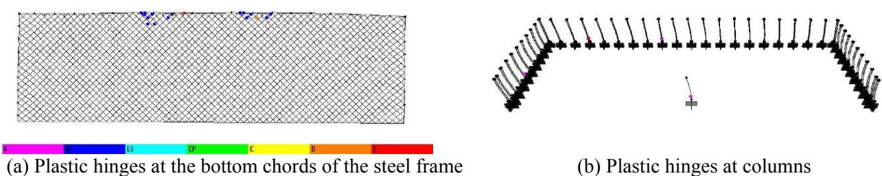
Fig.5 Plastic hinge distribution diagram from pushover analysis in *x* direction
