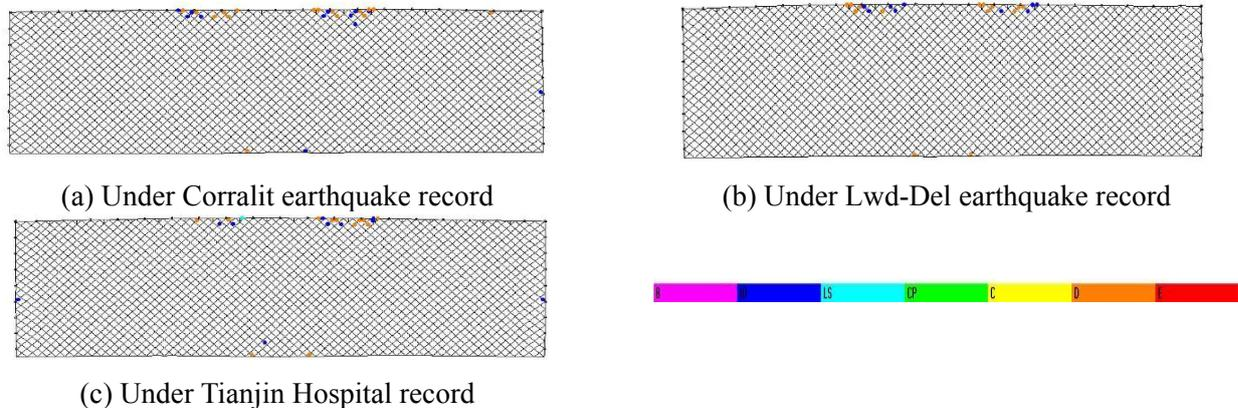
Fig.8 Plastic hinge distribution diagram of bottom chord members under severe earthquakes
