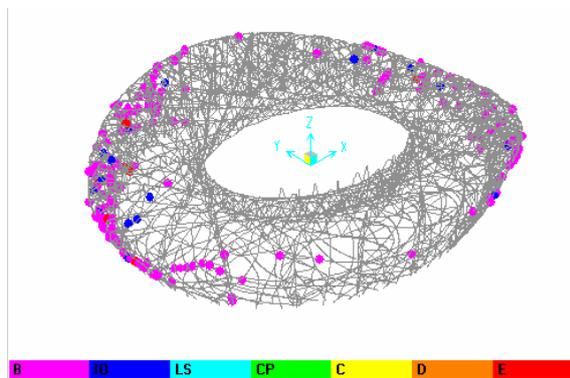
Fig.7 Plastic hinge location for pushover analysis case 11
