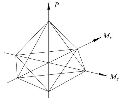
Fig.3 Sketch of yield surface of P-M-M hinges
