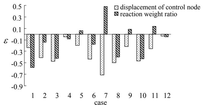
Fig.9 Relative errors between results of pushover analysis and dynamic analysis
