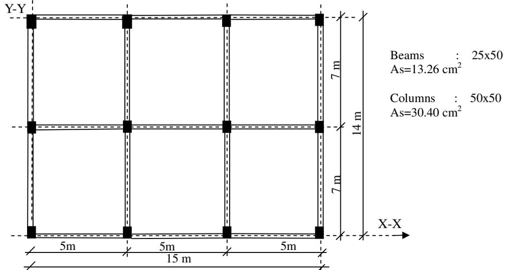
Figure 5. Plan view of the selected sample 4-story structure
