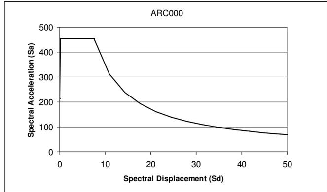
Figure 8. Idealized demand spectrum for Kocaeli, earthquake data (ARC000)
