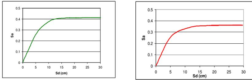
**a)** Capacity Spectrum in X-X      **b)** Capacity Spectrum in Y-Y
