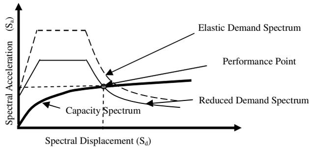
Figure 2 Determination of performance point by using previous methodology
