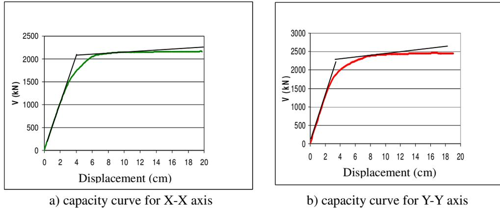
Figure 10 Idealization of capacity curves in displacement coefficient method
