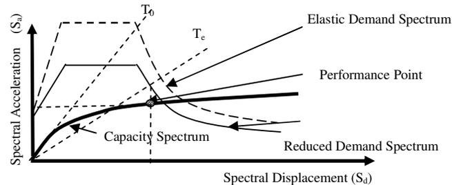
Figure 1 Determination of performance point by using new methodology
