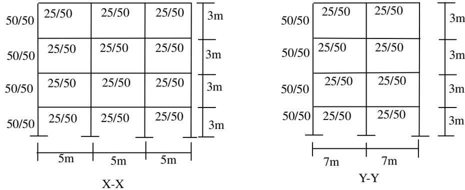
Figure 4 XX and YY Cross Sections of the sample 4-story structure
