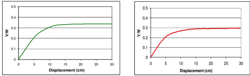
**a)** Capacity Curve in X-X      **b)** Capacity Curve in Y-Y
