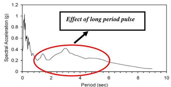
Figure 15 Spectral acceleration obtained by response analysis (Return period = 5000 year)
