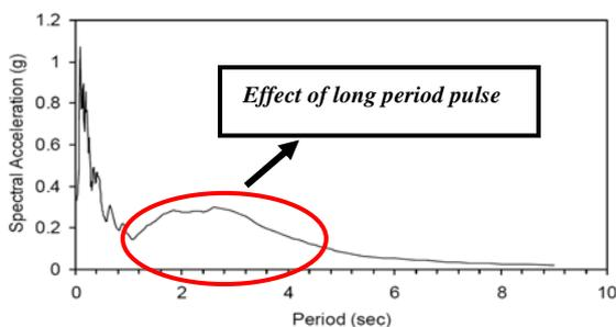
Figure 14 Spectral acceleration obtained by response analysis (Return period = 475 year)
