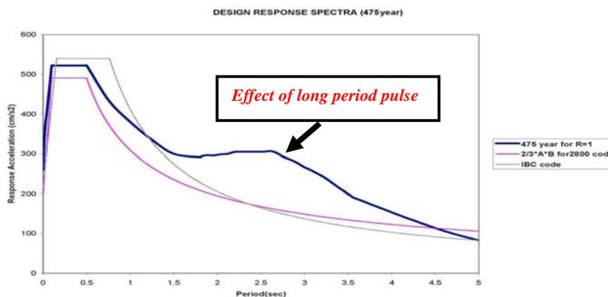
Figure 9 Comparison between response spectrums
