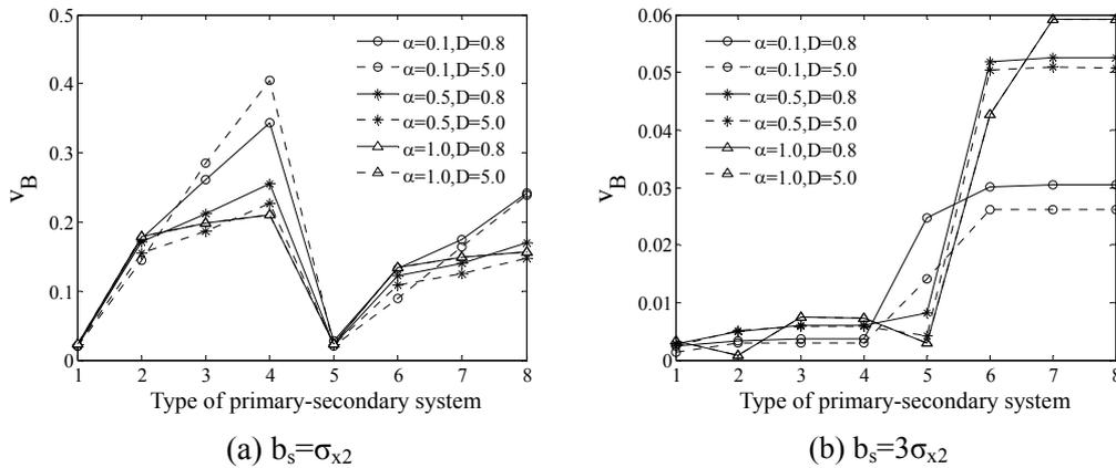
Figure 7 Effect of  $\alpha$  and  $D$  on crossing rate of primary-secondary systems
