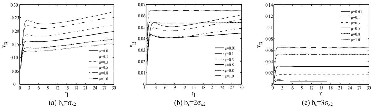
Figure 5 Effect of frequency ratio on the crossing rate of primary-secondary systems
