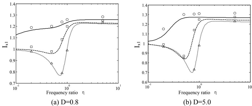
Figure 2 Amplification factor for variance of relative displacement of primary system with respect to the ground.  $\mu=0.1$ ,  $\zeta_p=0.05$ ,  $\zeta_s=0.05$ ,  $A=n=1$ ,  $\beta=0.05$ ,  $\gamma=0.95$ . —, Equivalent linearization,  $\circ$ , Moner Carlo, for  $\alpha=0.1$ ; - -, Equivalent linearization,  $\square$ , Moner Carlo simulation, for  $\alpha=0.5$ ; ---, Equivalent linearization,  $\Delta$ , Moner Carlo simulation, for  $\alpha=0.8$ .
