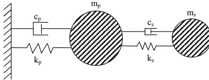
Figure1 Model of primary-secondary system
