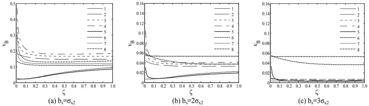
Figure 6 Effect of damping ratio on the crossing rate of primary-secondary systems
