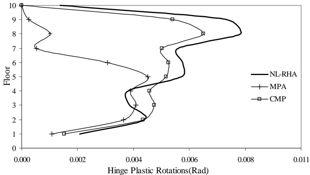
Figure 5 Height-wise variation of hinge plastic rotations for 10-storey frame
