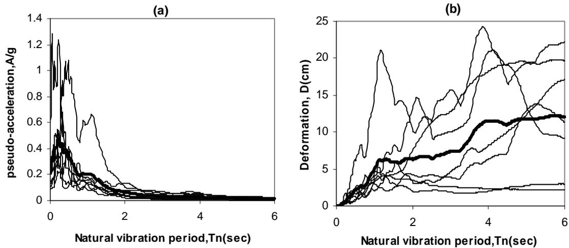
Figure 2 (a) Pseudo acceleration spectra and (b) displacement spectra of far field records set of ground motions, damping ratio=5%.
