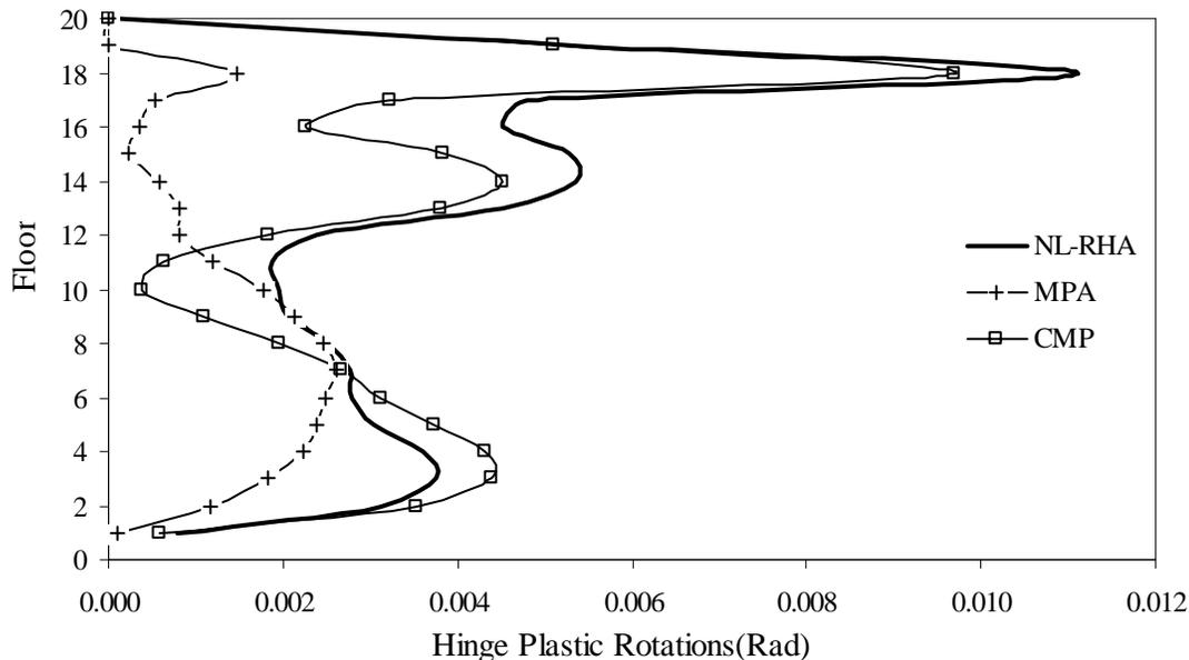
Figure 6 Height-wise variation of hinge plastic rotations for 20-storey frame
