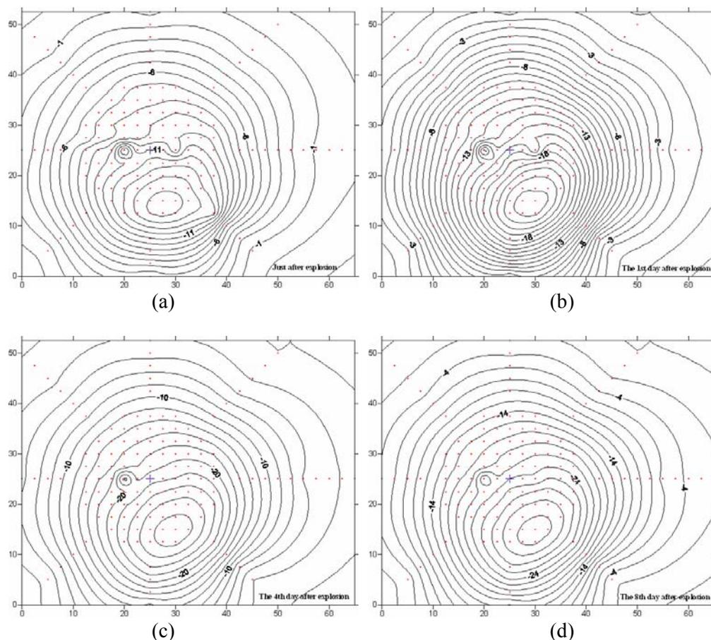
Figure 5 Isoline map of seismic subsidence of loess: (a) just after explosion, (b) the 1st day, (c) the 4th day, and (d) the 8th day, where the dots express the observation points of loess subsidence, and the cross is the center and subsidence unit is mm
