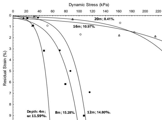
Figure 3 Characteristics of seismic subsidence of loess with different nature water content and depth
