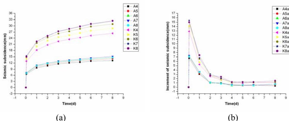
Figure 6 Developing process of seismic subsidence of loess with time, where A4~A8 and K4~K8 express the northmost and the southmost observation points respectively, and A4atb expresses the increment of loess subsidence at point A4 during one day
