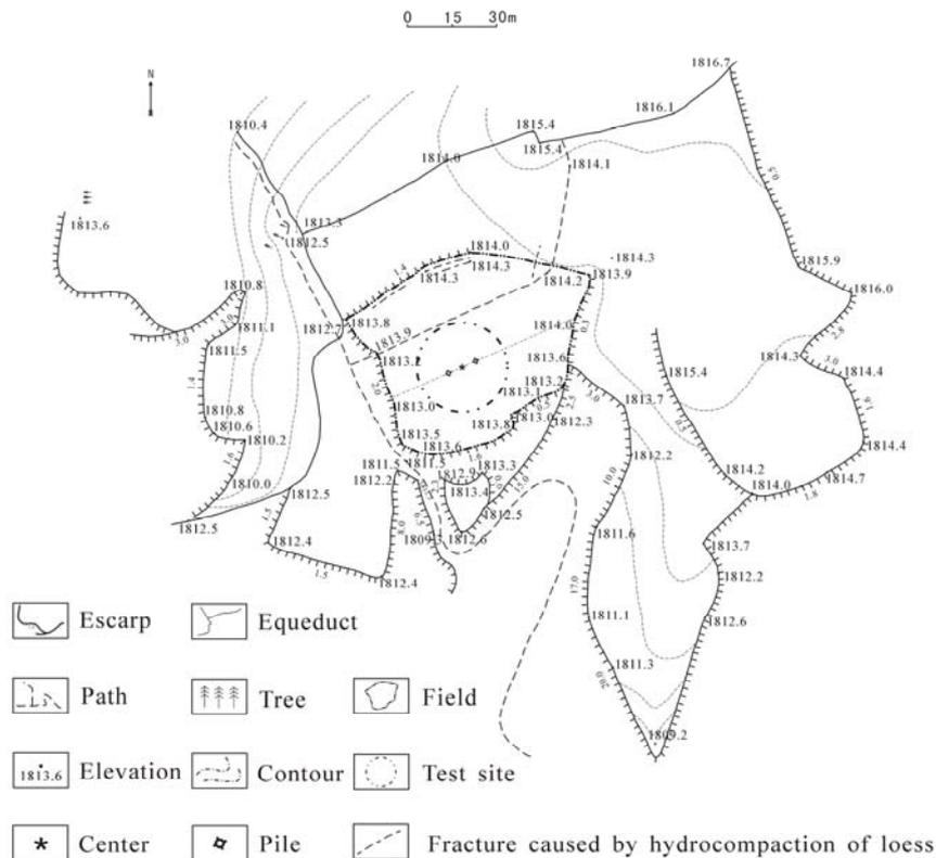
Figure 1 A rough drawing of landform around testing field
