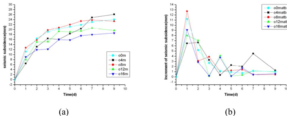
Figure 7 Variation of (a) seismic subsidence, and (b) settlement increment of loess layer with different depth, loess seismic subsidence at 0m represented by observation data of the center point on field surface
