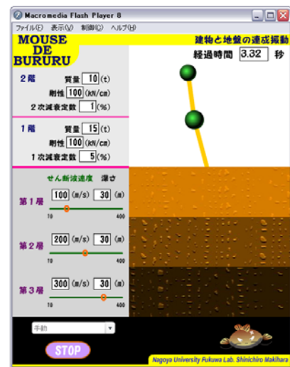
(d) Linear dynamic simulator for soil-layers and 2 stories structure system
