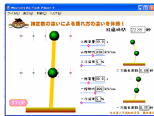
(a) Linear dynamic simulator for two DOF's system
