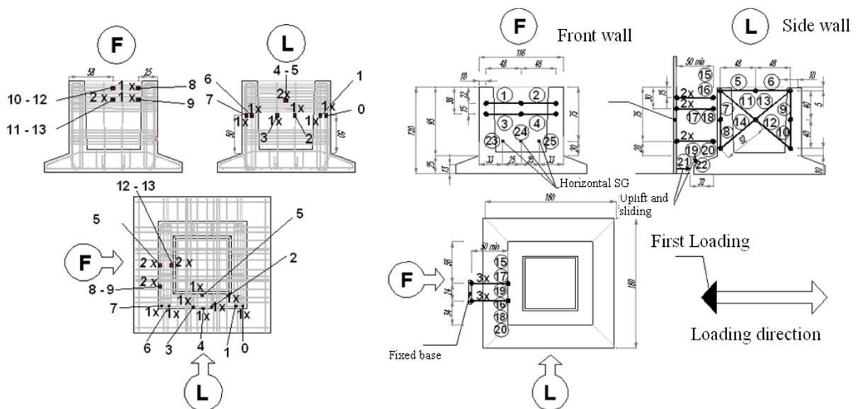
Figure 2.6 – Instrumentation of the column to foundation connections: strain-gauges (left); LVDT potentiometers (right)
