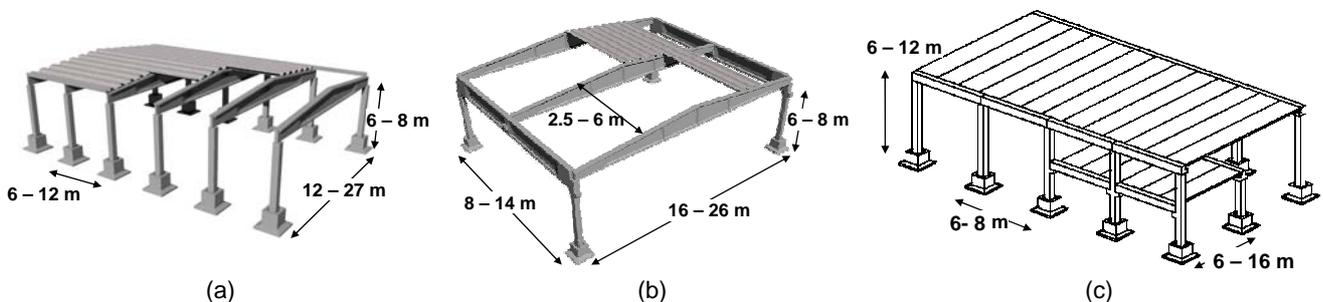
Figure 2.1 – Basic main structural typologies used in Italy: a) one-storey structure with portals; b) one-storey structure with portals and roof beams independent of the column grid; c) two- or three-storey structure.
