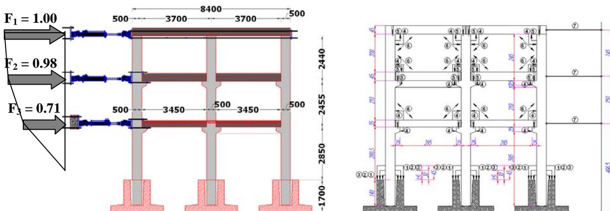
Figure 2.5 – Lateral force distribution (left) and instrumentation on the frame (right).
