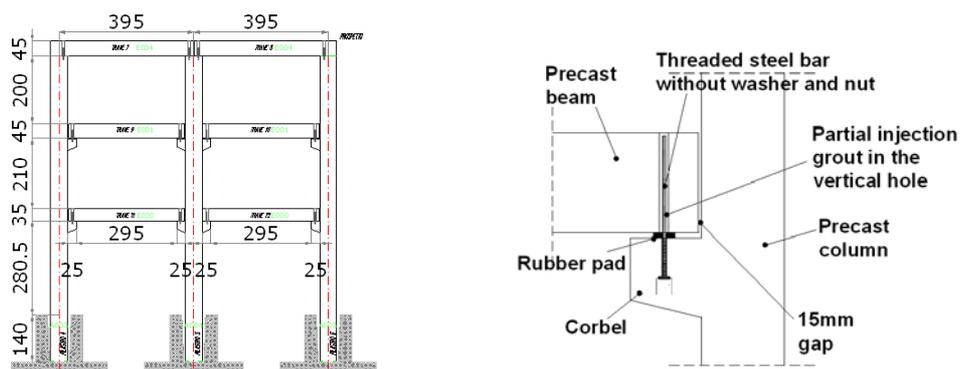
Figure 2.2 – Geometry of the specimen (left) and detail of the beam to corbel connection (right).
