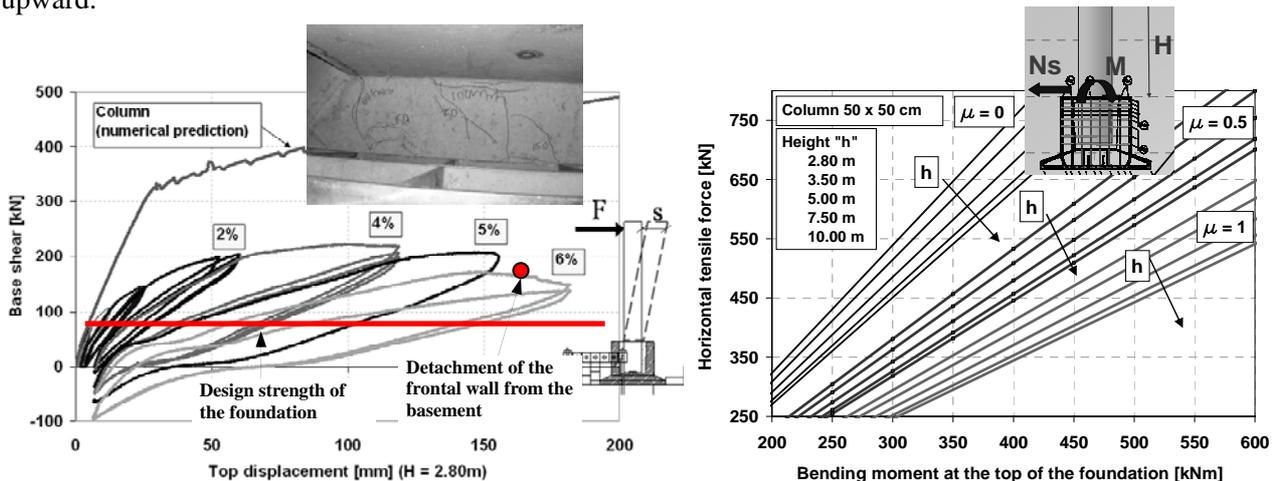
Figure 3.5 – Base shear – top displacement curve of the column of the socket foundation (left); cracking of the frontal wall of the foundation (top left); tensile force – bending moment curves as a function of the friction coefficient and of the height of the column (right)
