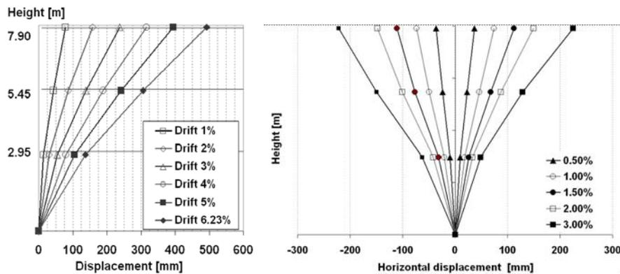
Figure 3.2 – Lateral deformed shape: numerical prediction (left); experimental result (right)
