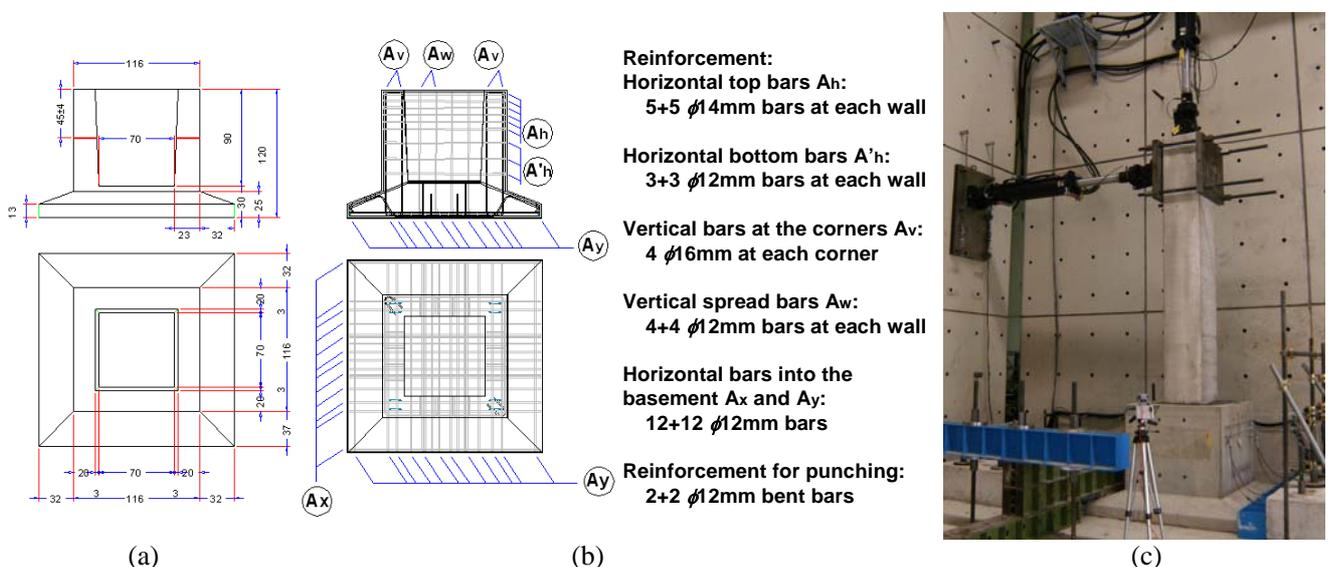
Figure 2.3 – (a) Geometry of the socket foundation; (b) details of the reinforcement; (c) test setup
