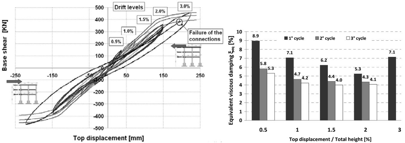
Figure 3.1 – Base shear – top displacement experimental curves (left); equivalent viscous damping (right)
