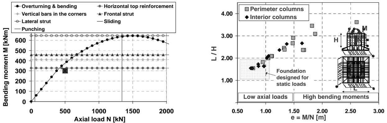
Figure 2.4 – Envelope of the design capacity domains of the specimens (left) and L/H ratio of socket foundation of three storey buildings as a function of the eccentricity of the seismic loads (PGA = 0.25g, Soil type C) (right).
