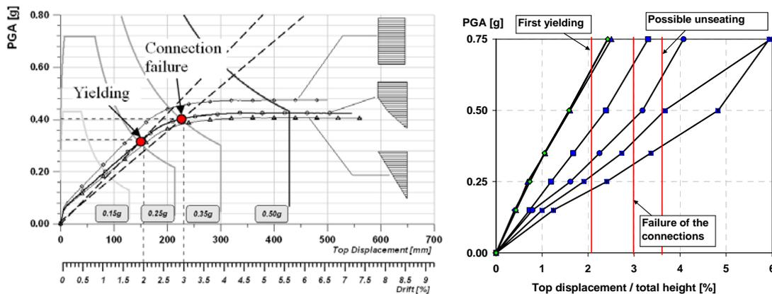
Figure 3.4 – Pushover curves for different lateral force profiles in the plane acceleration – displacement (left); acceleration – displacement curves obtained from the incremental dynamic analysis method with 7 accelerograms compatible with the spectrum defined in the Eurocode 8 for dense soil (right)
