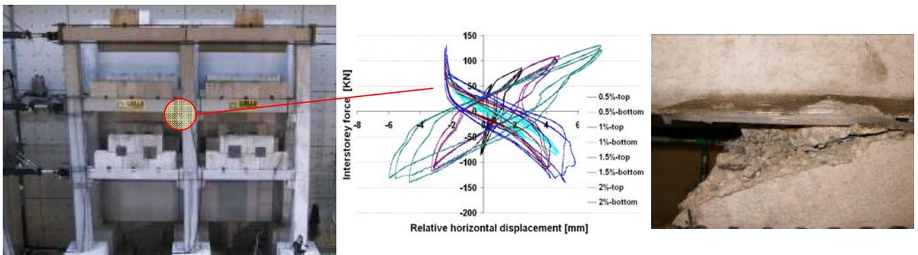
Figure 3.3 – Total lateral deformed shape during the test at drift 2% (left); expulsion of the concrete at a support (centre); interstorey shear – relative top and bottom horizontal displacement curves of a connection (right).
