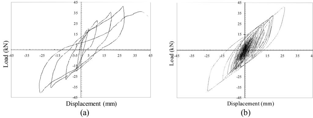
Figure 3. Experimental and fitted hysteresis loops for (a) Experimental test and (b) Model BWBN
