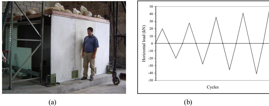
Figure 1. Experimental: (a) general view of test structure and (b) loading sequence
