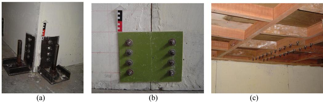
Figure 2. Details of integrity of the test structure: (a) support panels, (b) support between panels and (c) roof
