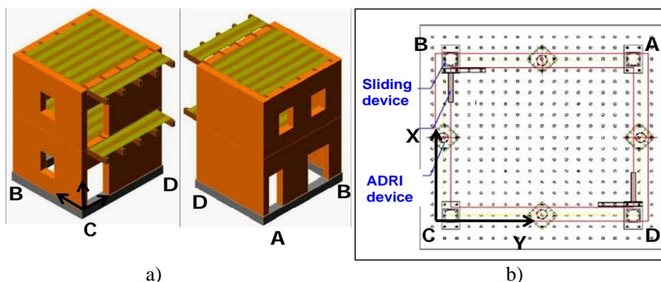
Figure 1. Geometry of both models (a), plans of isolation system.
