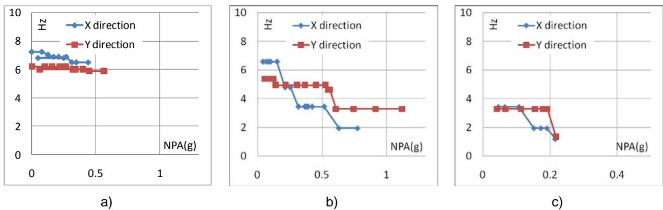
Figure 8. 1<sup>st</sup> structural frequency decay of model reinforced with a) ADRI, b) CAM and c) Fixed base, in both horizontal directions, the values are plotted vs the NPA.
