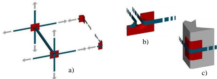
Figure 2. CAM system details: a) a typical setting; b) steel funnel shaped plate; c) angle plate
