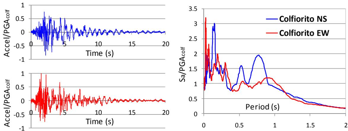
Figure 4. Colfiorito scaled accelerograms and corresponding 5% damping response spectra
