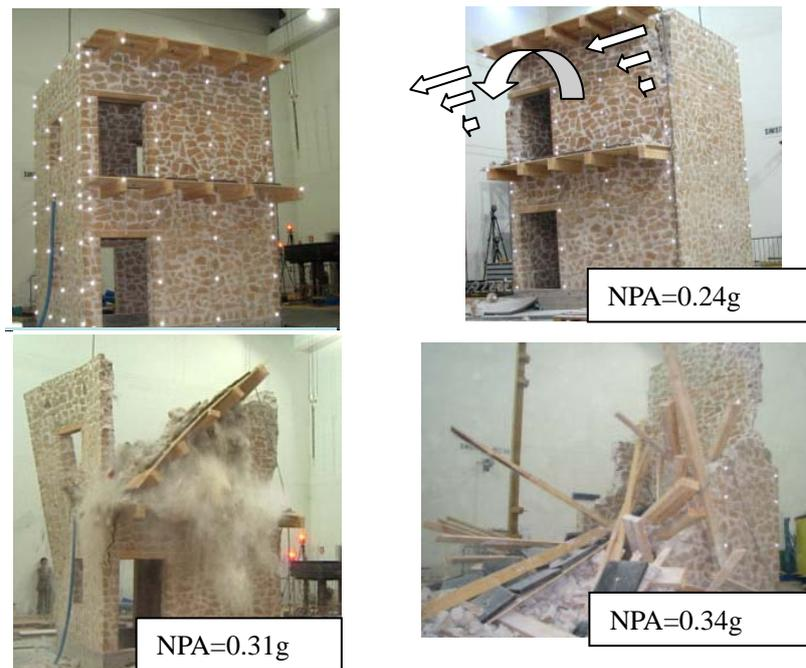
Figure 9 Model B collapse sequence
