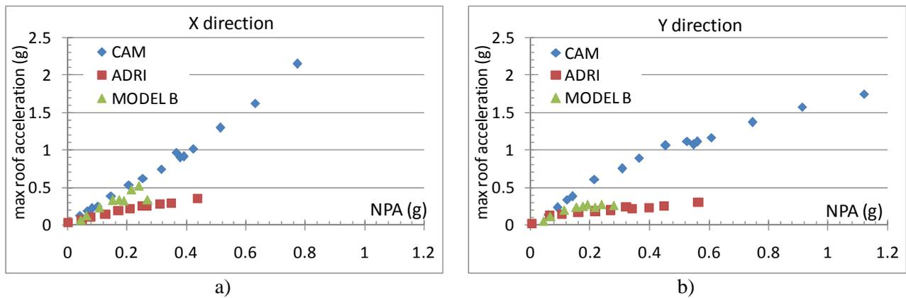
Figure 7. Max roof accelerations of model Vs NPA in X and Y direction.
