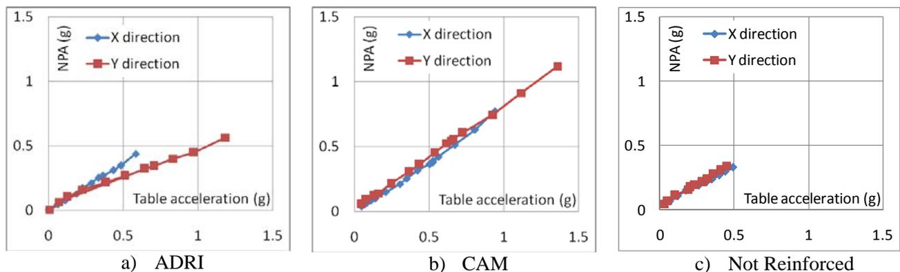
Figure 5. NPA Vs PGA in X and Y directions.
