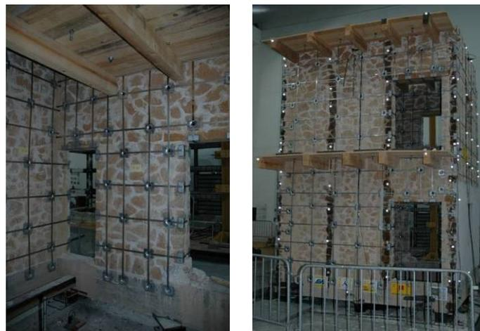
Figure 3. CAM system reinforced model
