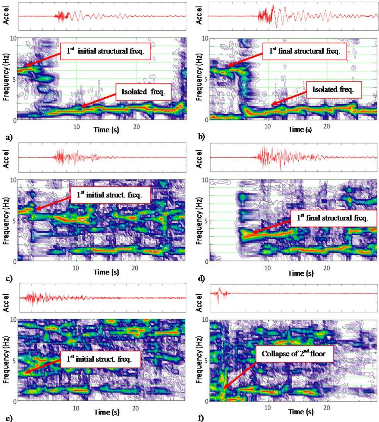
Figure 6. Spectrograms Model A: ADRI, a) 0.162g NPA test, b) 0.56 NPA test g - Model A: CAM c) 0.216 NPA test, d) 1.129g NPA test - Model B: No reinforced e) 0.043g NPA test, f) 0.31g NPA test
