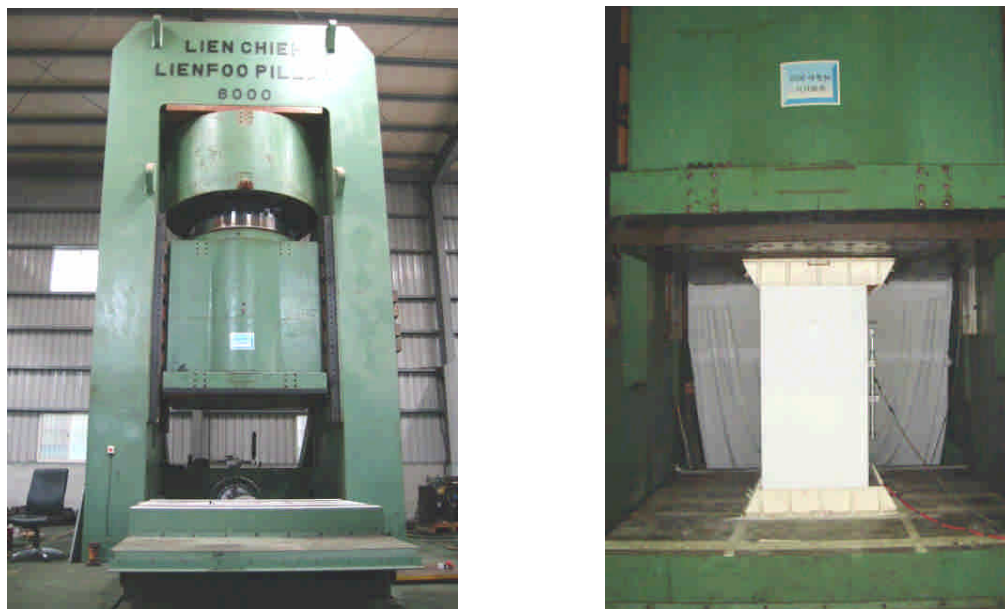
Fig. 3 The 58800 kN test machine and the set-up of the test
