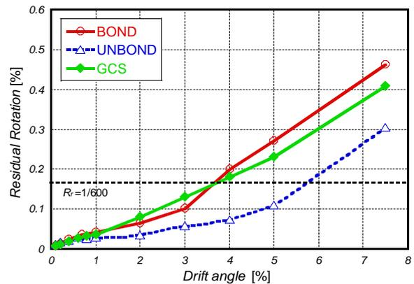
Figure 13 Residual drift angles
