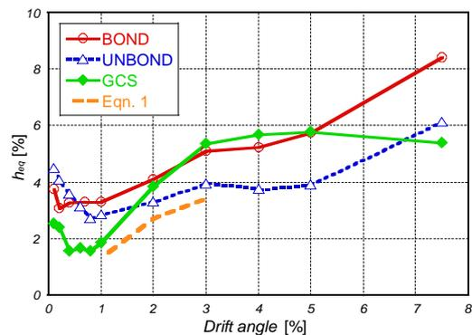
Figure 12 Equivalent viscous damping ratios
