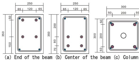
Figure 6 Cross sections of specimens (unit: mm)
