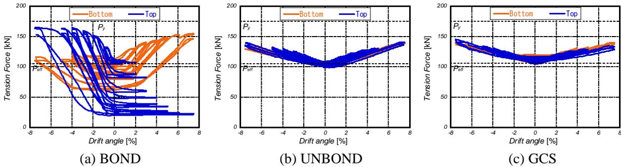
Figure 11 Tensile force of prestressing bars and strands (beam)
