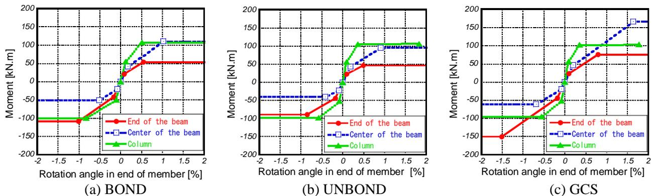
Figure 15 Restoring force characteristic in ends of members
