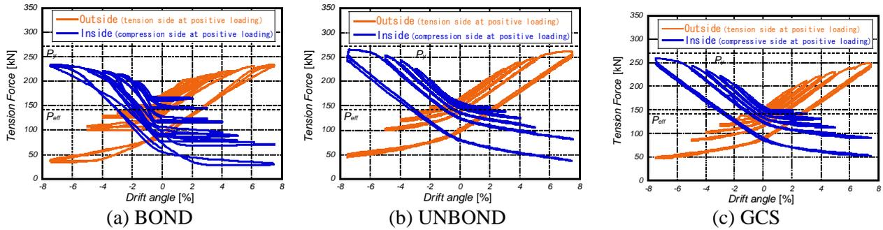
Figure 10 Tensile force of prestressing bars and strands (column)
