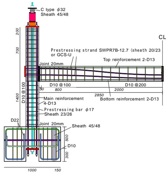
Figure 5 Specimen dimensions (unit: mm)
