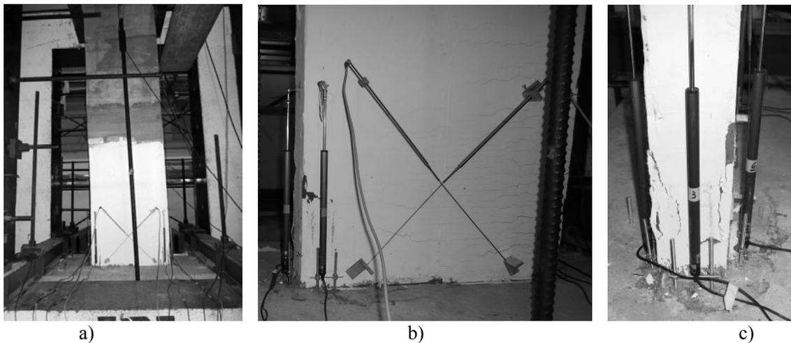
Figure 5. a) Side view of the deformed shear wall at collapse; b) detail of the crack pattern in the critical zone; c) collapse induced by the crushing of the jacket.
