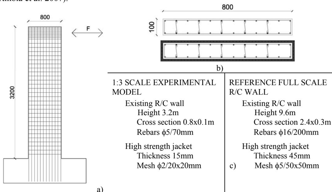
Figure 2. a) Front view and b) cross section of the experimental model; c) geometric properties of the 1:3 scaled model and the full scale reference R/C wall.
