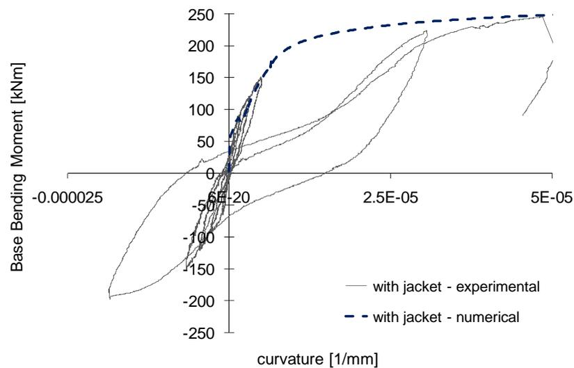
Figure 6. Bending moment versus curvature experimental curve for the strengthened shear wall and numerical response for the unreinforced R/C wall.
