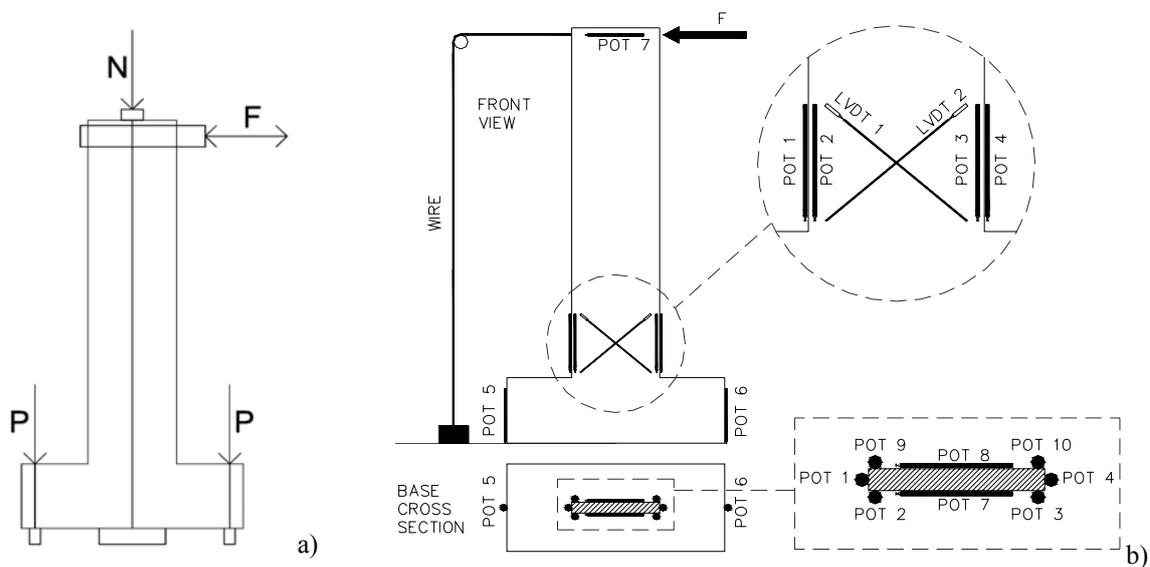
Figure 3. a) Scheme of the loading modalities; b) instrument set up.
