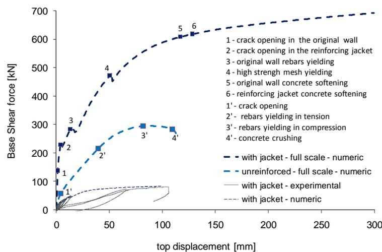
Figure 7. Full scale model: applied horizontal load versus top displacement curve.
