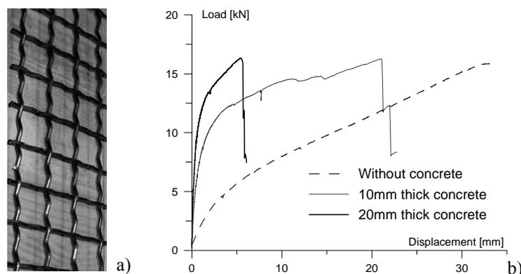
Figure 1. a) High strength steel mesh made of bent wires; b) tensile tests performed on the bare high strength steel mesh and on specimens made of high strength steel mesh embedded in 10 and 20mm high performance concrete layers.
