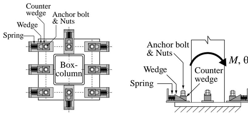
(a) Arrangement of Wedge device on base plate
