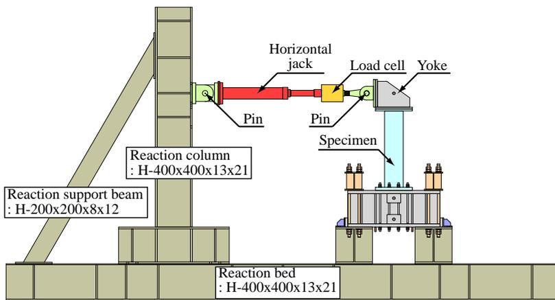
Figure 3 Apparatus
