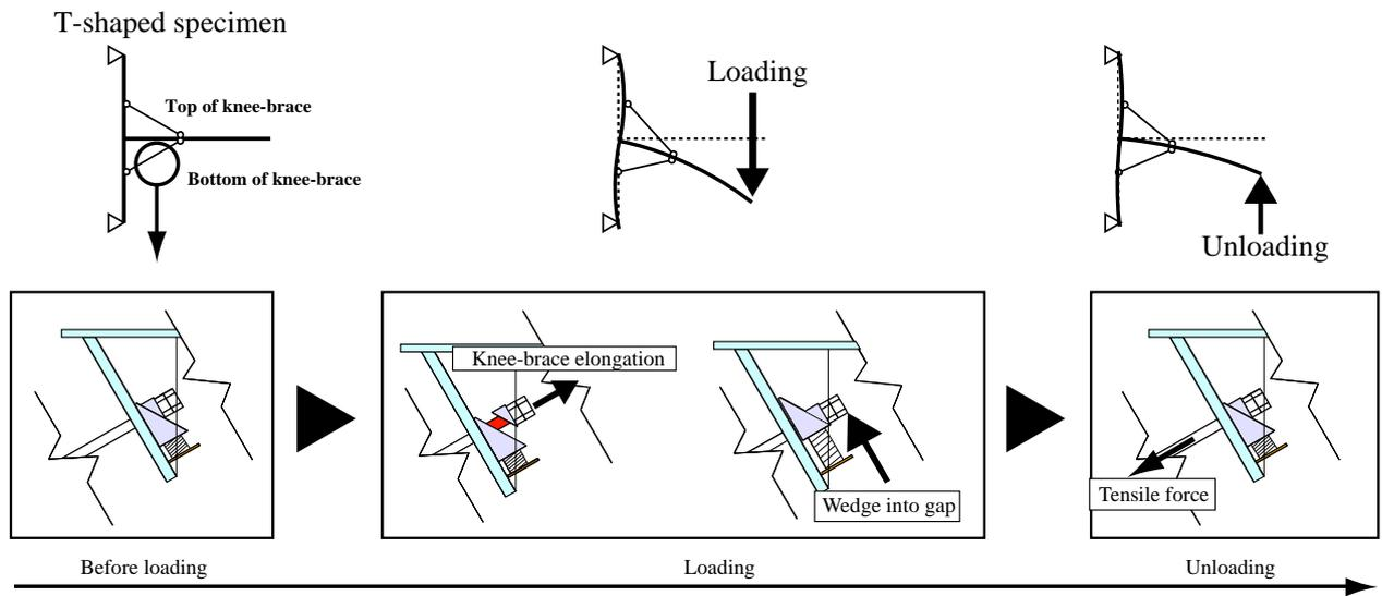
Figure 17 Function of non-compression knee-brace
