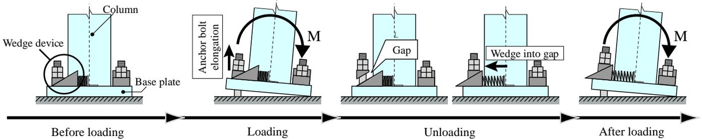
Figure 1 Function of non-slip-type column-base
