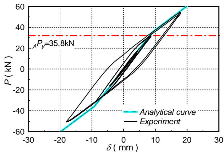
Figure 20 Horizontal load v.s. Horizontal displacement relations
