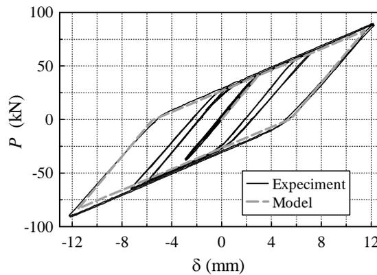
Figure 10 Horizontal load v.s. Horizontal displacement relations
