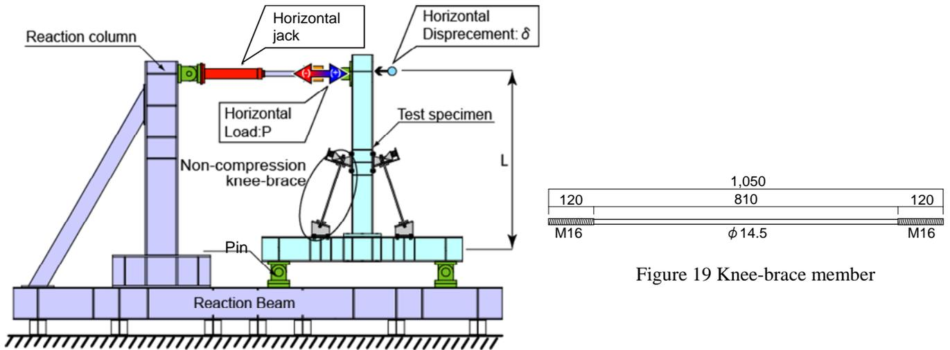
Figure 18 Apparatus
