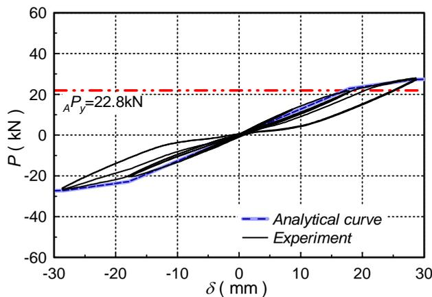
Figure 15 Horizontal load v.s. Horizontal displacement relations
