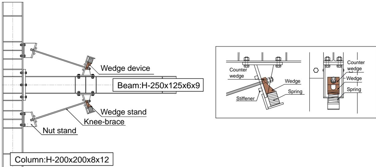
(a) Arrangement of wedge device on knee-brace end
