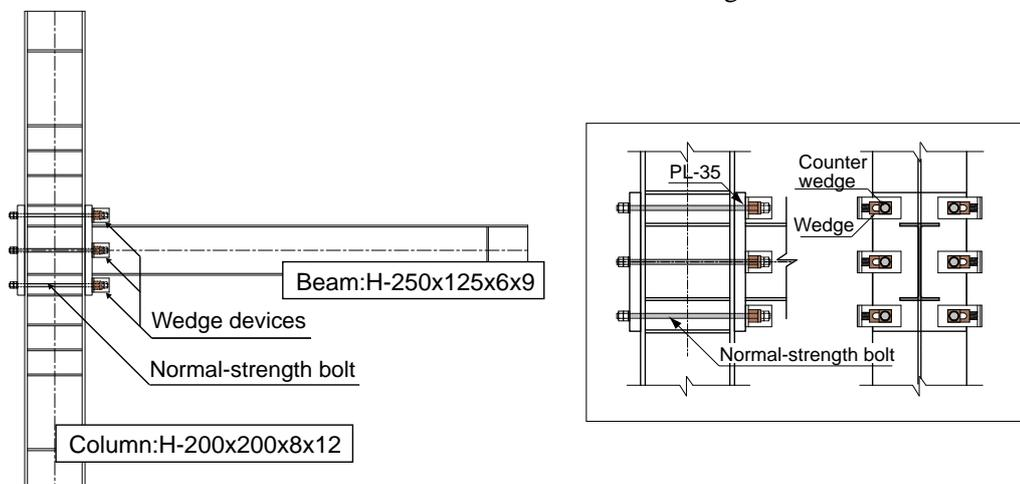
(a) Arrangement of wedge device on end-plate
