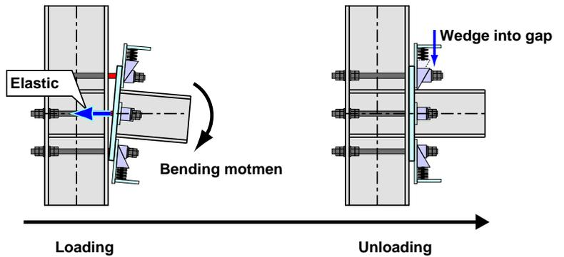
Figure 12 Function of self-centering connection
