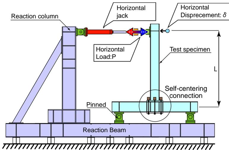
Figure 13 Apparatus
