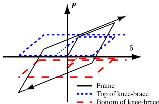
(b) Model of restoring force characteristics
