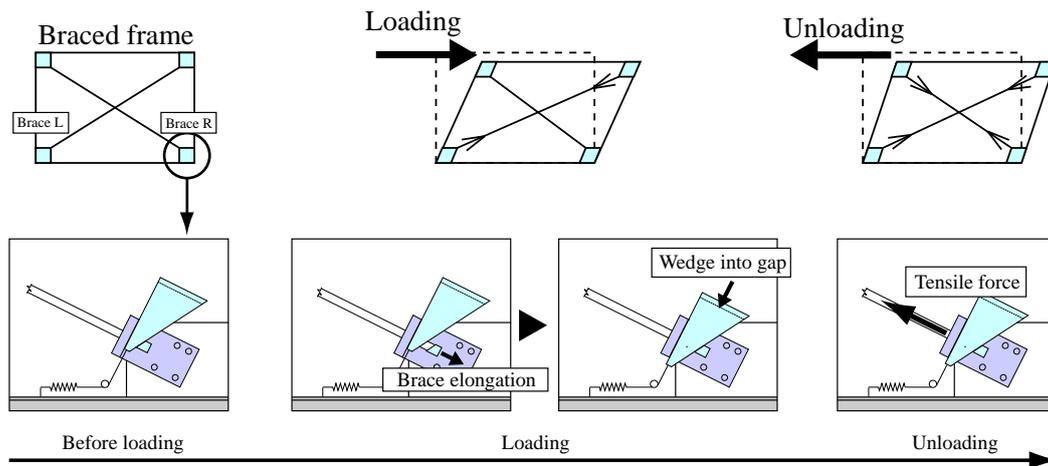
Figure 7 Function of non-compression brace
