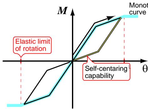
(b) Model of restoring force characteristics
