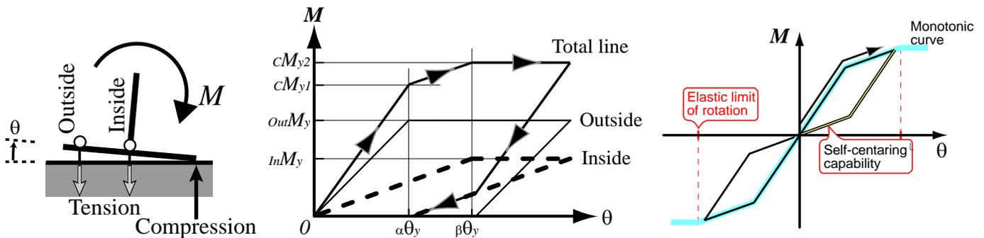
(b) Resistant mechanism and model under monotonic loading
