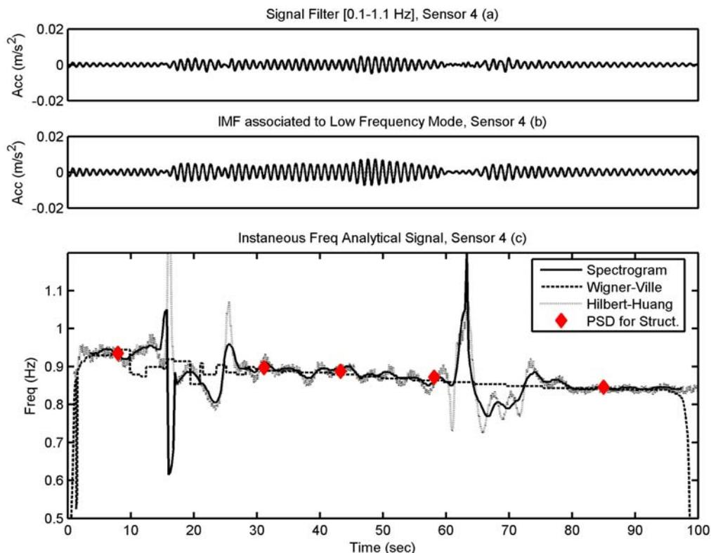
Figure 10: a) Filter Recorded Acceleration. B). IMF associated with low frequency and C) Comparison of Estimates for Predominant Frequency as a Function of Time using Spectrogram, HHT, WVD also shown with red diamonds the values obtained from PSD study with the arm at the different fix extensions.
