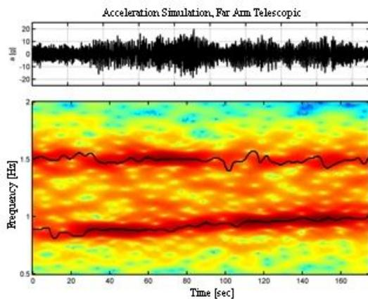
Figure 12: Spectrogram telescopic end arm signal, analytic simplified Model.
