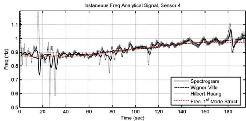
Figure 15: Estimated predominant frequency as a function of time using spectrogram, HHT, WVD for the idialized model.
