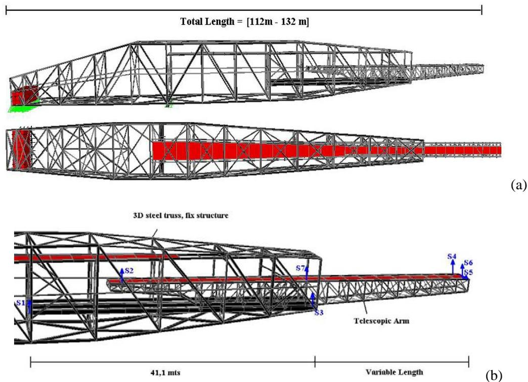
Figure 1: (a) 3-D Structure, (b) Sensor Location.
