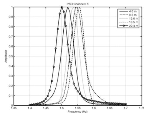
Figure 3: Power Spectral Density Frequency Variation as a Function of Position. Higher Frequency. Sensor 6.
