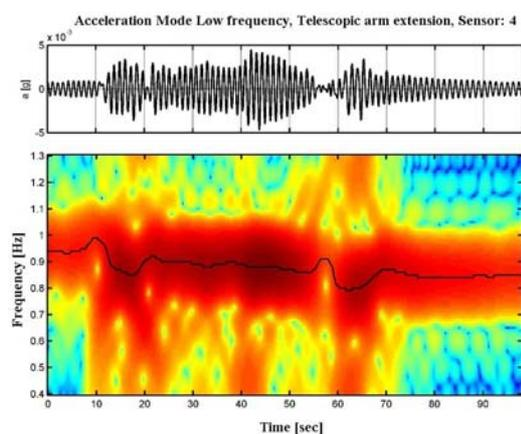
Figure 5: Spectrogram Vertical Acceleration, Sensor 4. Telescopic Arm Extension. LF.
