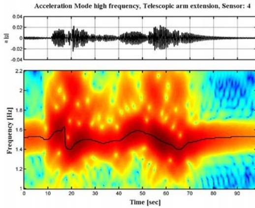
Figure 6: Spectrogram of Vertical Acceleration of Sensor 4. Telescopic Arm Extension. HF.
