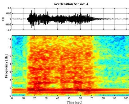
Figure 4: Spectrogram Vertical Acceleration, Sensor 4. Telescopic Arm Extension.
