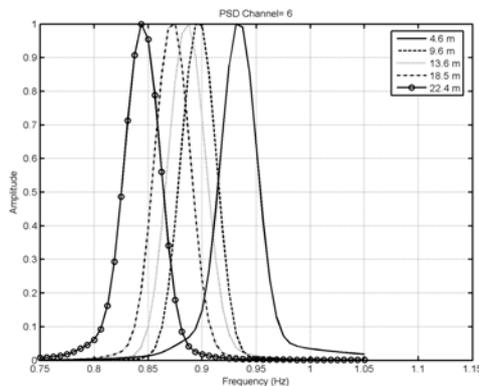
Figure 2: Power Spectral Density Frequency Variation as a Function of Position. Lower Frequency. Sensor 6.
