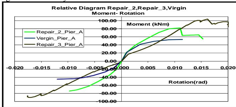
Figure 17b. Flexural response of repaired Rep-3, Rep-2 and virgin specimens.
