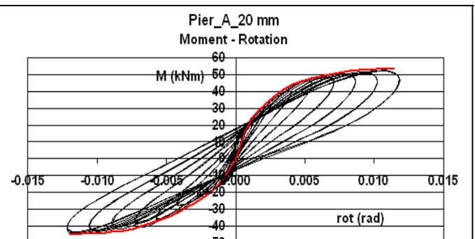
**Figure 6b.** The measured flexural response of Pier A in terms of bending moment - plastic rotation.
