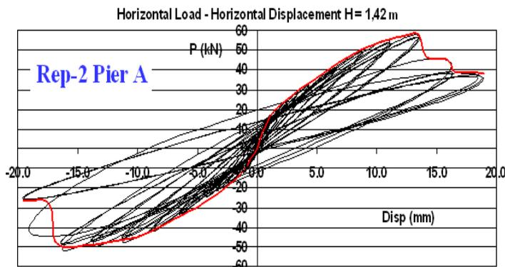
**Figure 10a.** The measured flexural response of Rep-2 Pier A in terms of horizontal load - horizontal Displacement.
