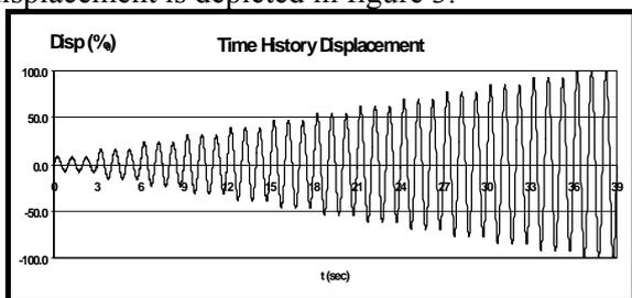
Figure 3. Imposed horizontal displacement
