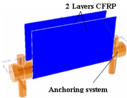
Figure 13a. New anchoring device
