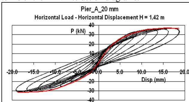
**Figure 6a.** The measured flexural response of Pier A in terms of horizontal load - horizontal Displacement
