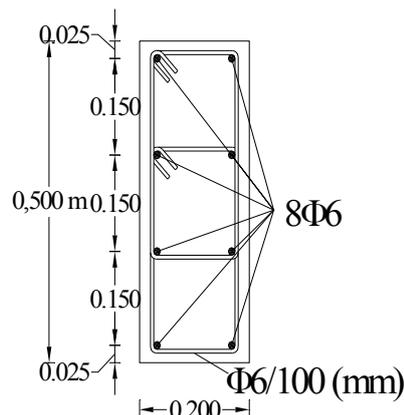
Figure 2b. Cross-section and reinforcing details of Pier A
