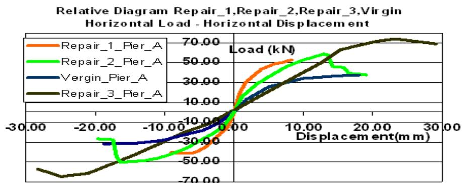
Figure 17a. Flexural response of repaired specimens Rep-3, Rep-2, Rep-1 and virgin specimen.
