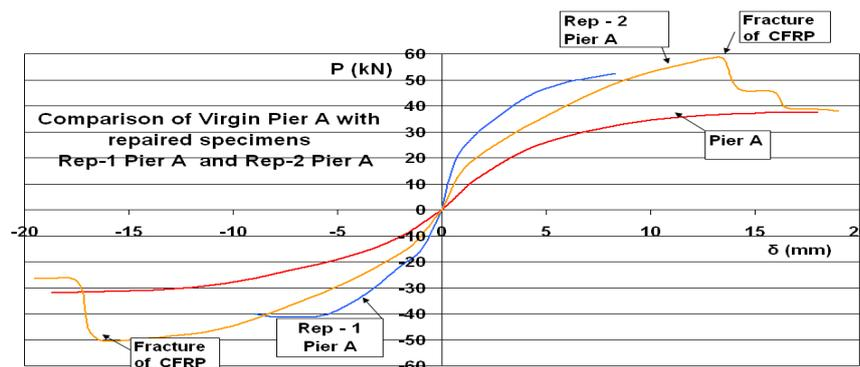
**Figure 11.** Comparison of flexural response of repaired Rep-2 Pier A with repaired specimen Rep-1 Pier A and virgin specimen Pier A in terms of Horizontal load – Horizontal displacements.
