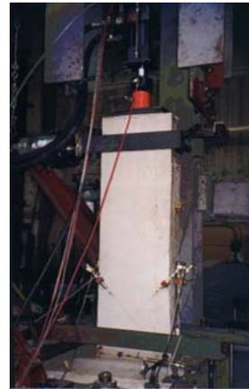
**Figure 5.** Pier A placed at the strong reaction frame
