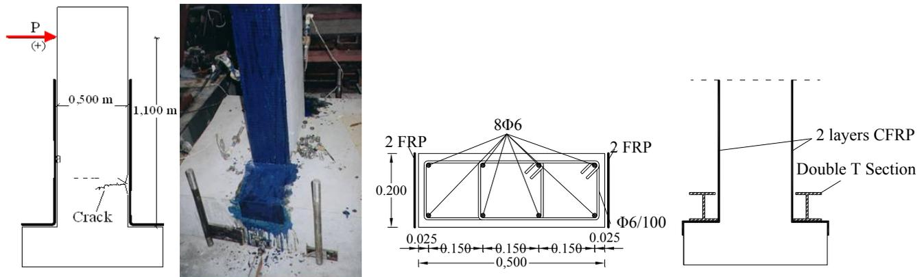
Figure 7. Details for specimen Rep-1 Pier A
