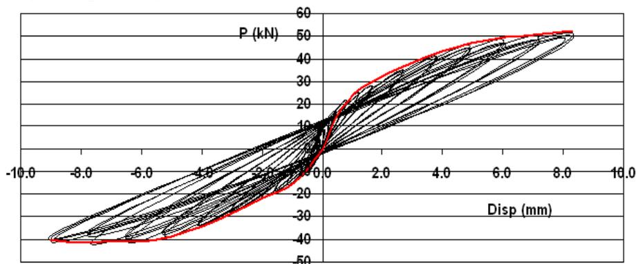
Figure 8. The measured flexural response of Rep-1 Pier A in terms of Horiz. load – Horiz. Displacement.
