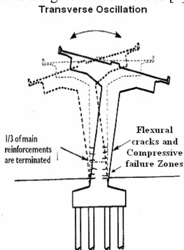
Figure 1. Flexural Damage
