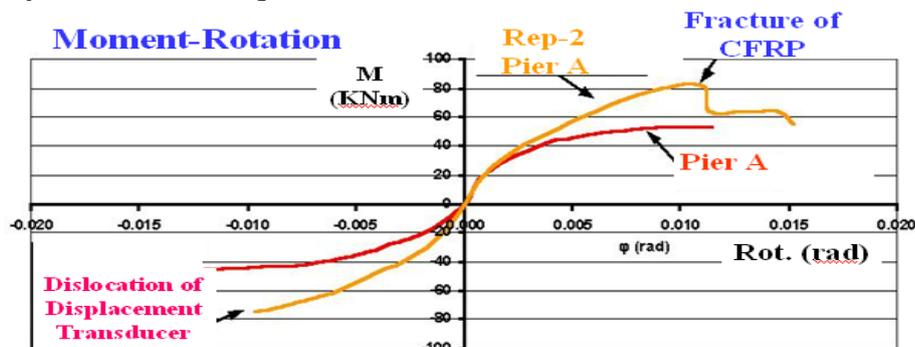
**Figure 12.** Comparison of flexural response of repaired Rep-2 Pier A with virgin specimen Pier A
