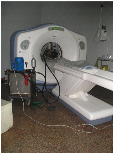
Figure 3 The portable test device to fitting medical CT scanner
