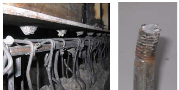
Fig 4 Fractured Studs on Upper Interface of Second Story
