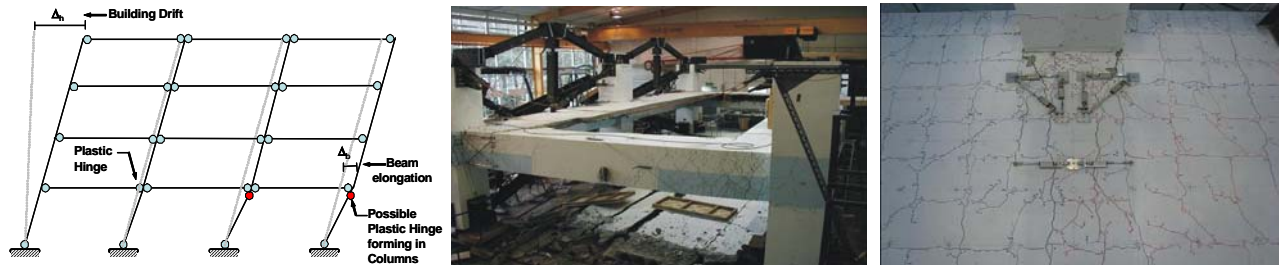
Figure 1 Desirable weak beam strong column mechanism (Left); Floor collapse due to lost of floor support (Centre) [Matthews et al., 2003]; Floor slab crack patterns (Right). [Peng et al., 2008].
