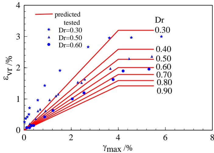
Fig.9 Sand-gravel post-liquefaction volumetric strain plotted against maximum shear strain
