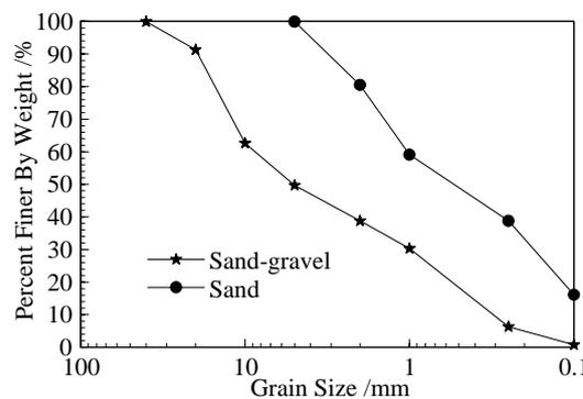
Figure 1 Grain Size Distribution Curves for Tested Materials
