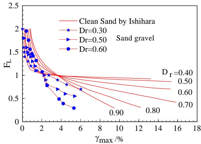
Fig. 10 Relation of factor of safety and maximum shear strain of sand and sand-gravel
