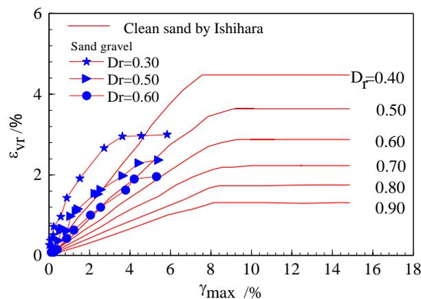
**Fig.8** Sand and sand-gravel post-liquefaction volumetric strain plotted against maximum shear strain
