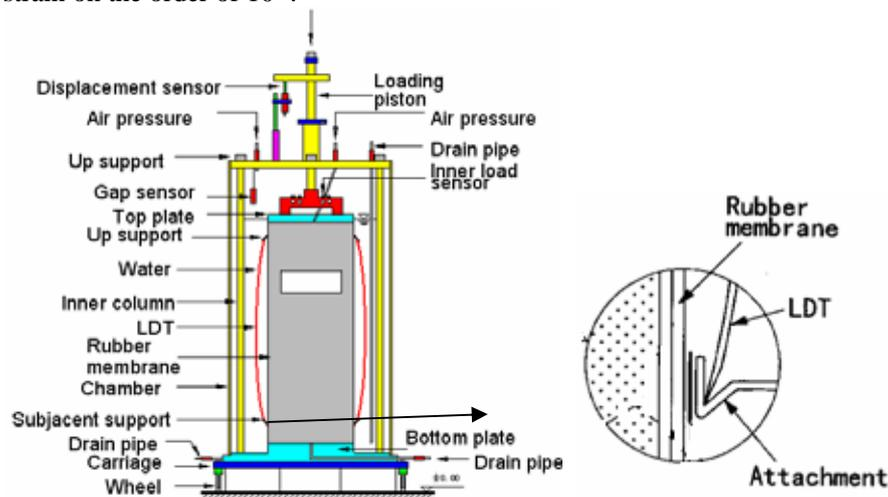
Figure 2 Triaxial test device
