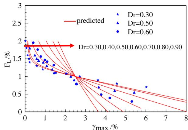
**Fig. 11** Relation of factor of safety and maximum shear strain of sand-gravel
