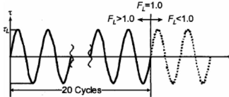
Fig.3 Schematic diagram of  $F_L$  definition
