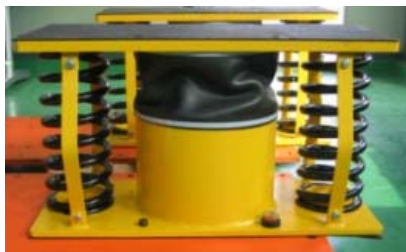
Figure 2 Spring-damper unit for the EDG test model
