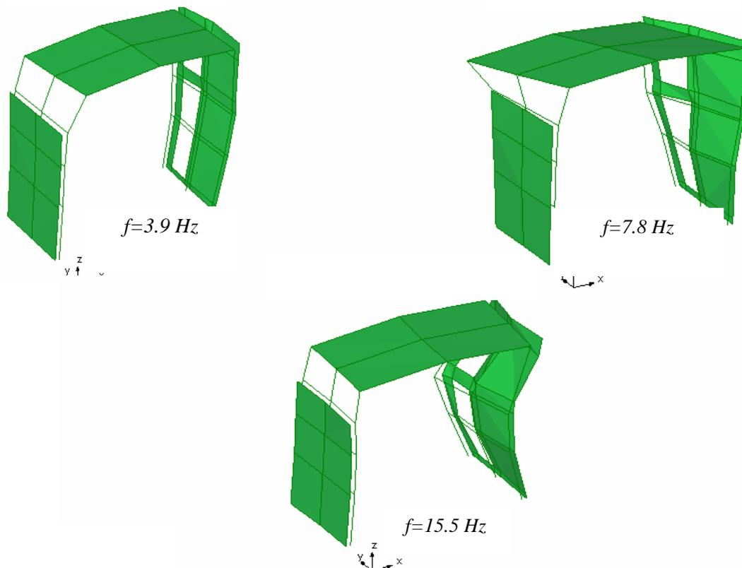
Figure 9 Mode shapes of vibration for the model
