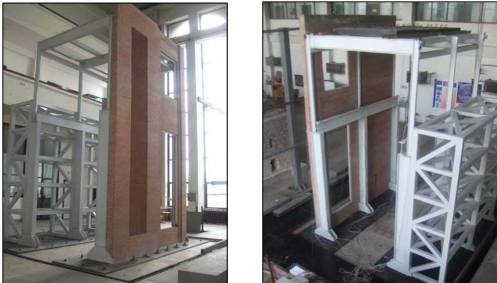
Figure 7 The model of the wall ready for shaking table testing
