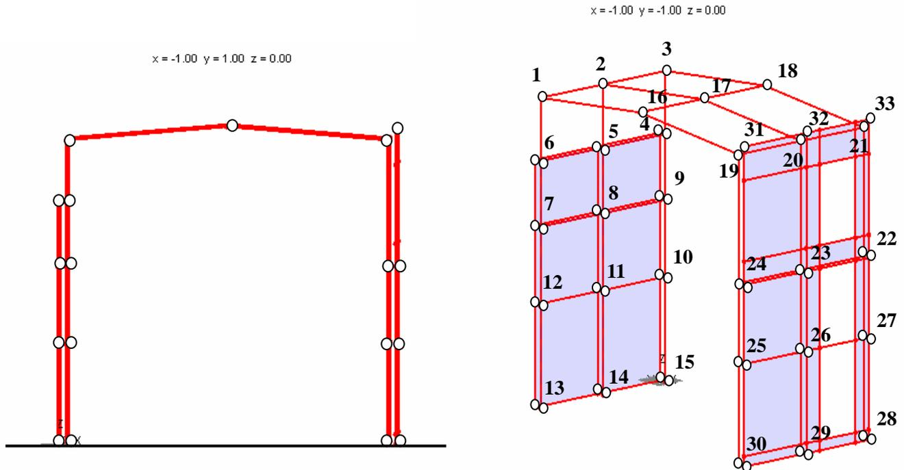
Figure 3 Measuring points on the selected portion of the Beauharnois powerhouse
