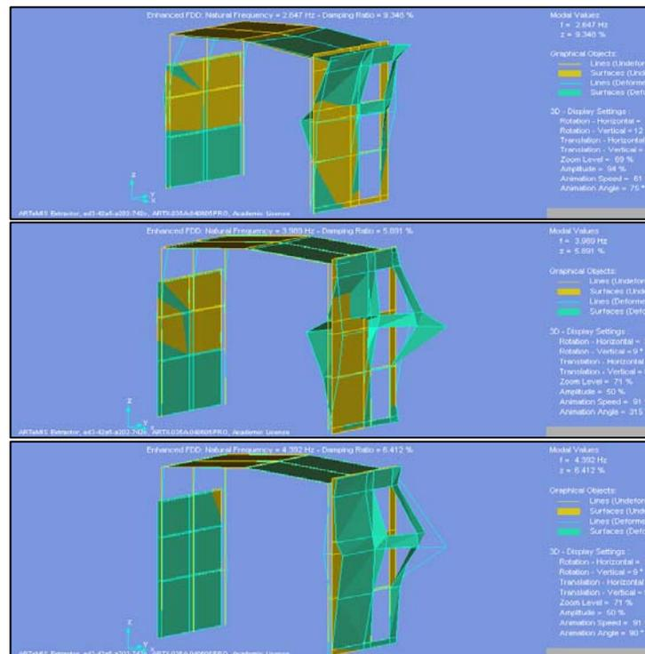
Figure 5 Mode shapes of vibration for the first three frequencies
