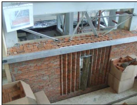
Figure 6 The model of the wall under construction
