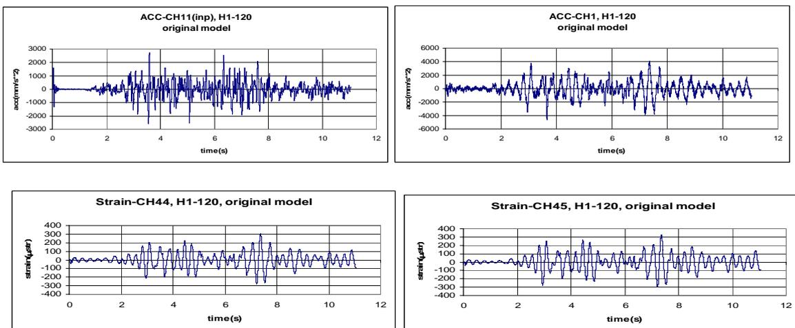
Figure 11 Selected time histories for the maximum expected earthquake intensity of 0.2g
