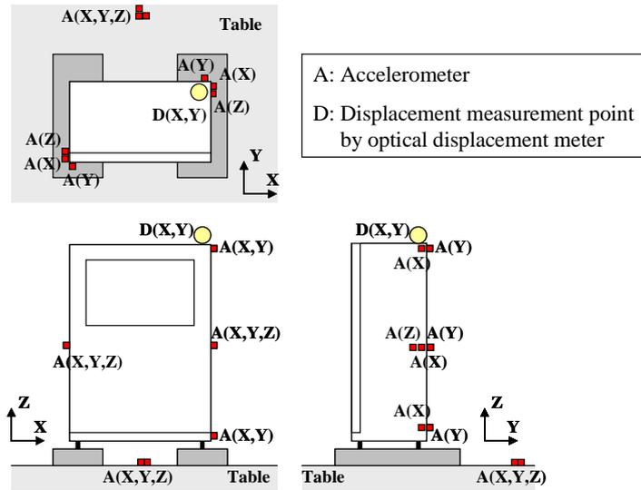
Figure 4 The measurement point
