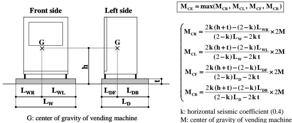
Figure 2 Specification of required mass in JIS
