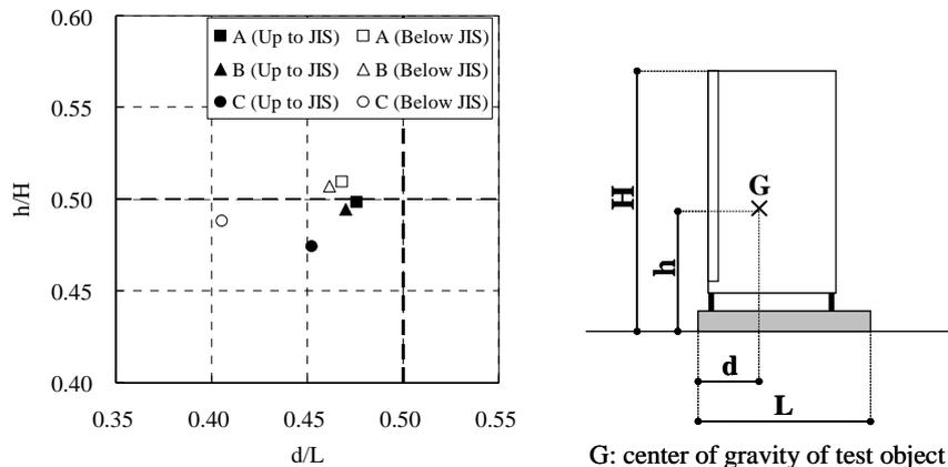
Figure 3 Center of gravity of each test object
