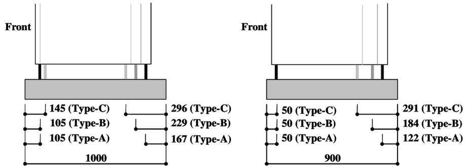
Figure 2 Position of vending machine on blocks
