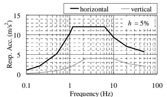
Figure 5 Target response spectra for ART-JIS
