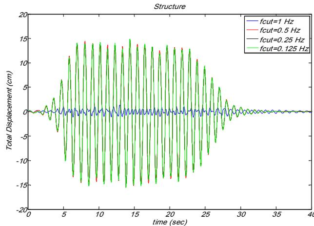
Figure 5. Diaphragm displacement time histories. Maximum input acceleration = 0,21g
