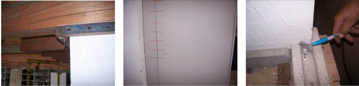
(a) No damage at the diaphragm level (b) No damage between panels (c) Spalling at the tip due to rocking
