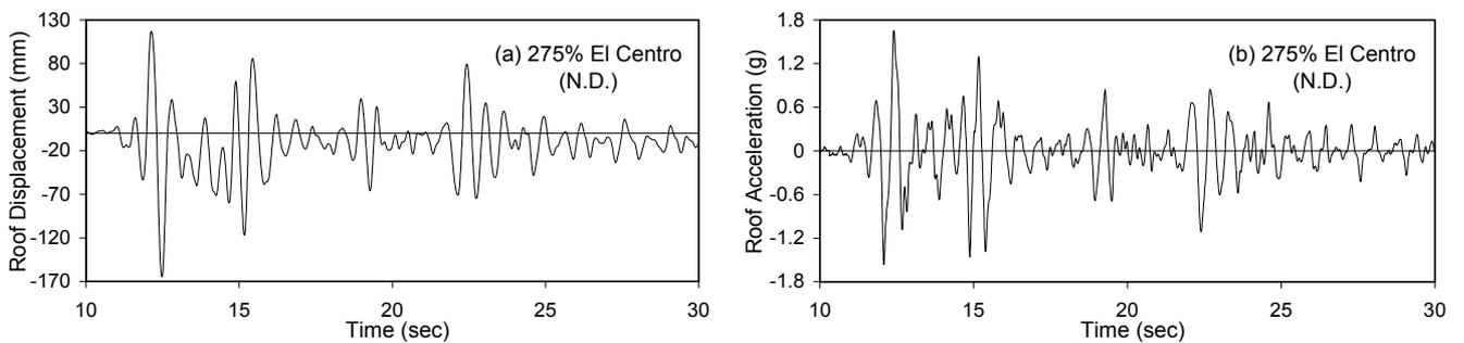
Fig.6. Roof lateral (a) displacement and (b) acceleration of retrofitted structure under 275% El Centro earthquake.
