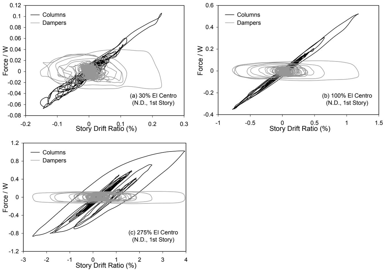
Fig.5. Column shear and damper force at the first story under various earthquakes.
