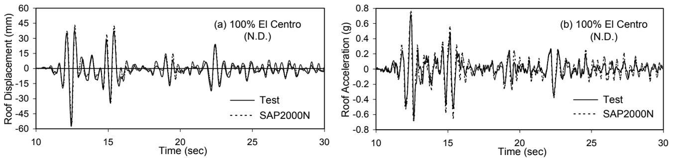
Fig.8. Simulation of (a) roof displacement and (b) roof acceleration for retrofitted structure under 100% El Centro earthquake.
