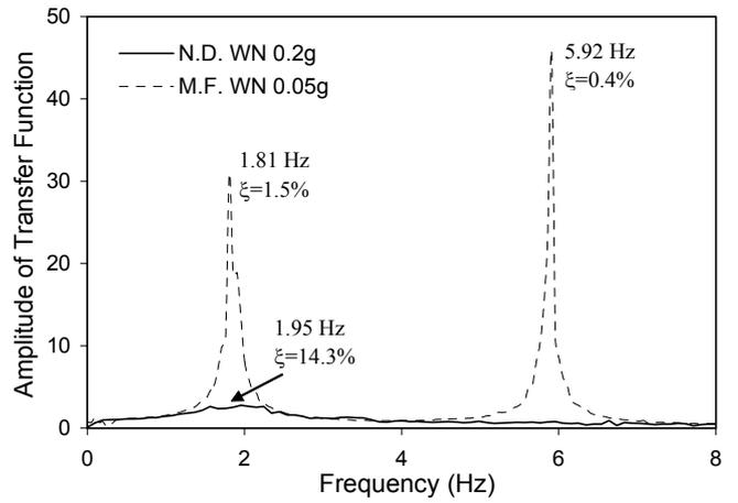
Fig.2. Transfer functions for structures with and without dampers.
