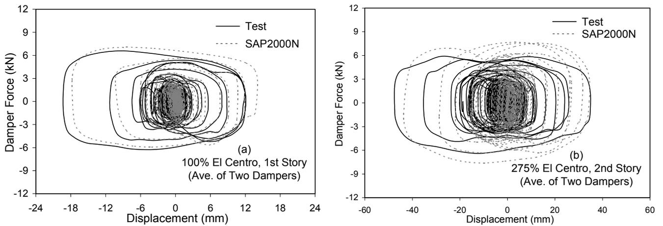
Fig.7. Simulation of damper force at the 1st story under (a) 100% and (b) 275% El Centro earthquakes.
