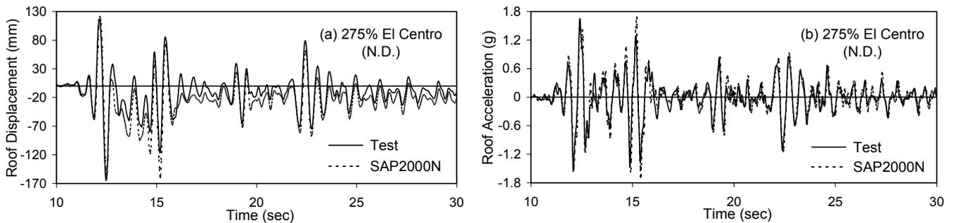
Fig.9. Simulation of (a) roof displacement and (b) roof acceleration for retrofitted structure under 275% El Centro earthquake.
