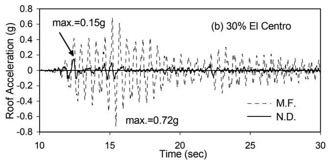
Fig.4. Roof lateral (a) displacement and (b) acceleration under 30% El Centro earthquake.
