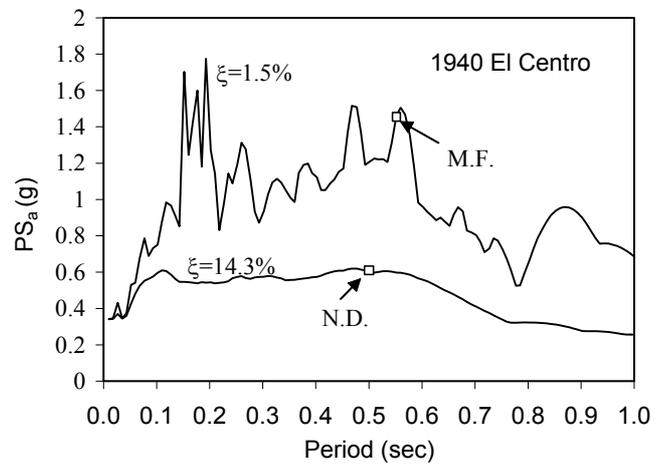
Fig.3. Response spectra of 1940 El Centro Earthquake.
