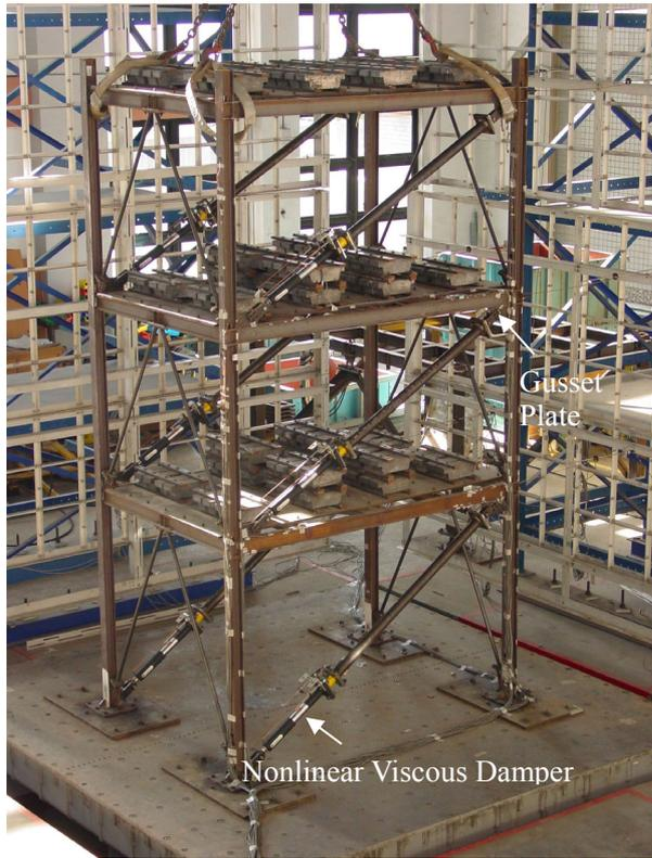
Fig.1. Layout of 2/3-scale 3-story test structure.
