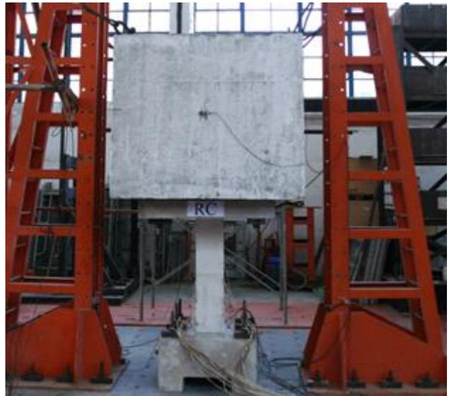
(b) Detail of configuration (c) Photo of test specimen on shaking table
