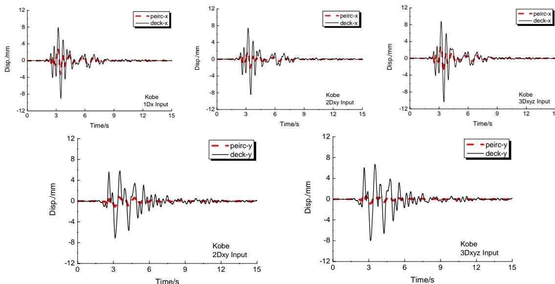
Figure 4 Displacement time history curve under multi-directional earthquake input ( Kobe,peak acceleration:0.4g)
