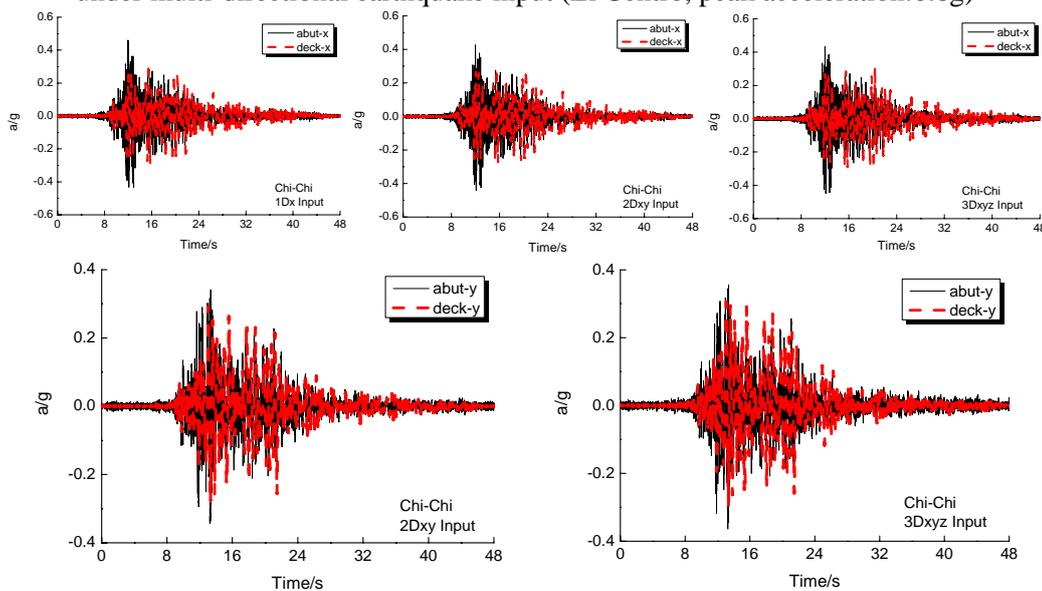
Figure3 Acceleration time history curve of pier and corresponding deck under multi-directional earthquake input (Chi-Chi, peak acceleration:0.4g)
