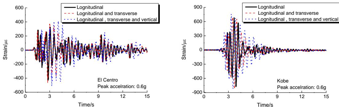
Figure7 Axial strain time history curve under multi-directional earthquake input
