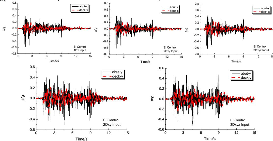
Figure 2 Acceleration time history curve of pier and corresponding deck under multi-directional earthquake input (El Centro, peak acceleration:0.6g)
