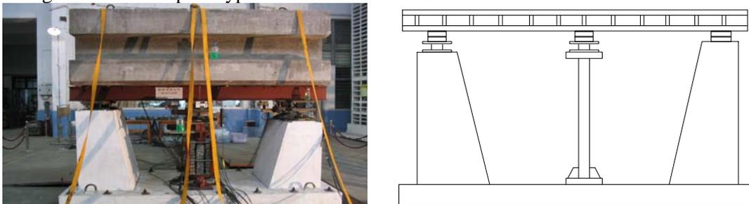
Figure1 The 1/10 isolated bridge model
