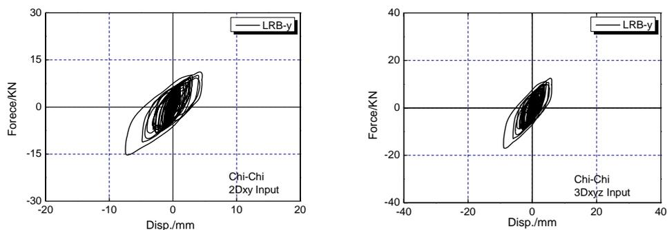
Figure 5 Force-displacement relationship curve in multi-directional Chi-Chi earthquake wave input
