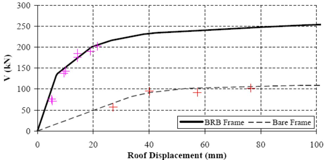
Figure 4. Seismic Demand for Bare Frame and BRB Frame
