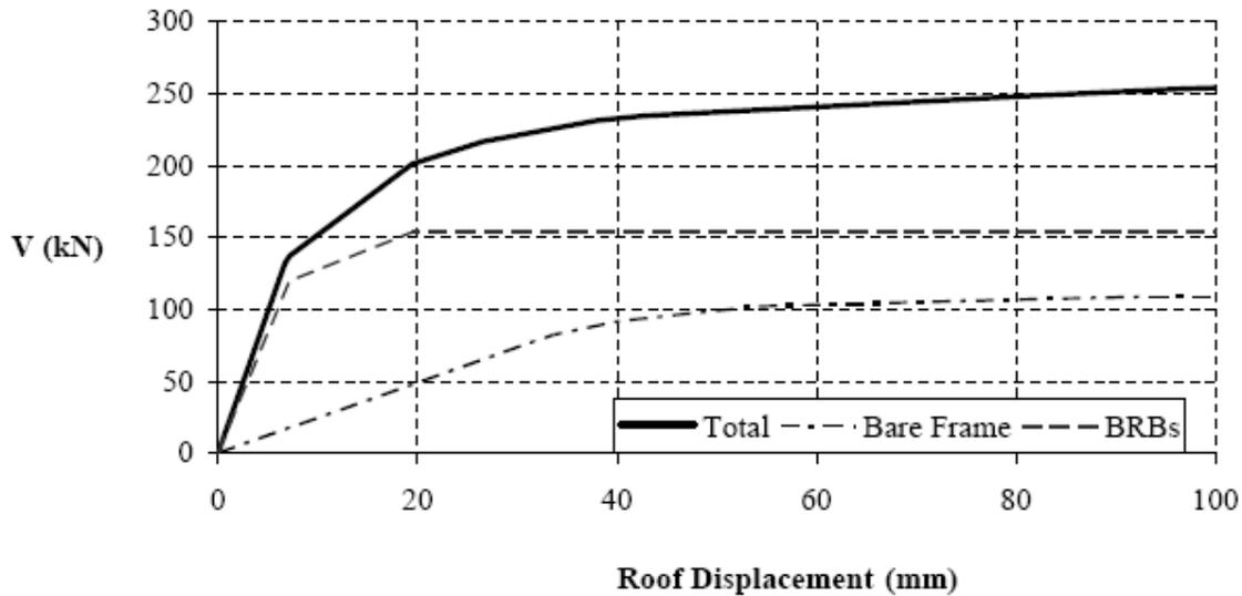
Figure 2. Pushover Curve for the Model
