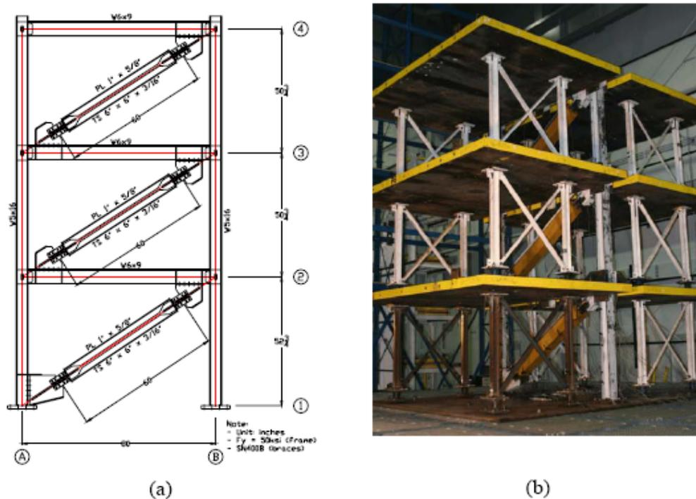
Figure 1. Experiment Setup: (a) Frame with Nippon Steel BRBs, (b) General View of the Experiment
