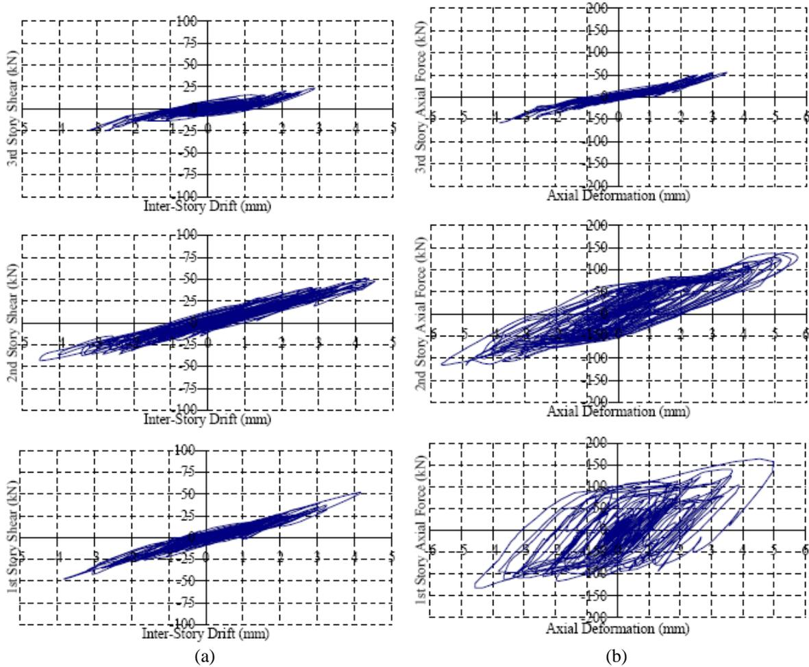
Figure 5. Hysteretic Response: (a) Columns Story Shear; (b) BRBs Hysteresis Loops
