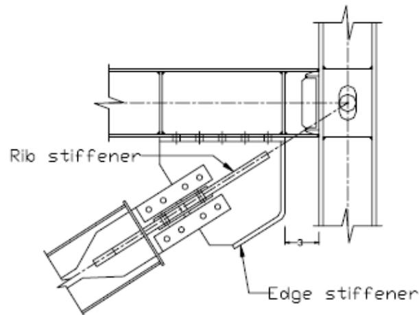
Figure 3. Typical Gusset plate details
