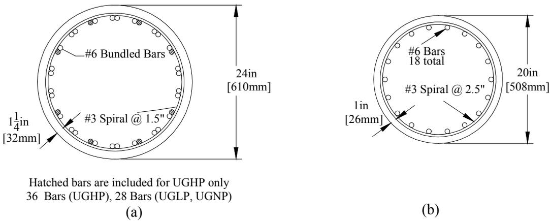
Figure 4: (a) Column section UGHP, UGLP, UGNP; (b) UGHPM
