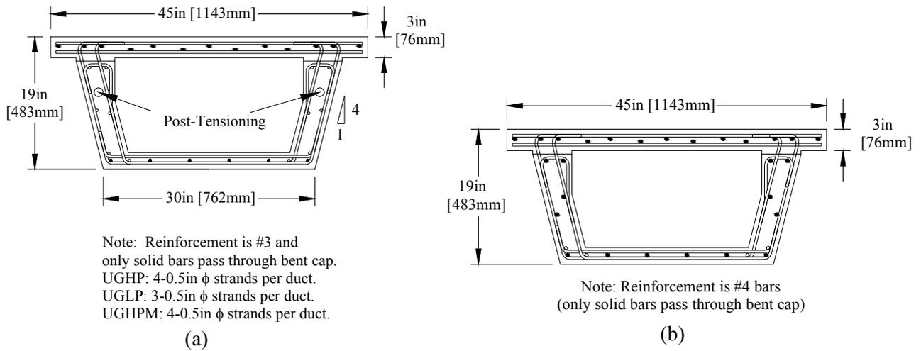
Figure 3: a) Girder section UGHP, UGLP, UGHPM; (b) UGNP
