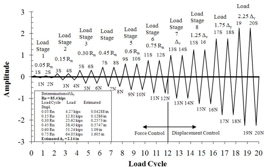
Figure 2: UGHP Reverse Cyclic Lateral Loading Protocol
