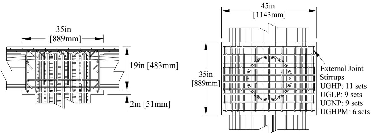
Figure 5: Joint Reinforcement
