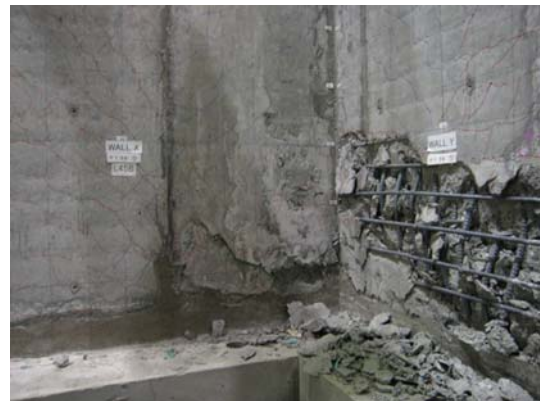
Figure 6 Lateral load – drift angle relations and pictures of the specimens after the loading
