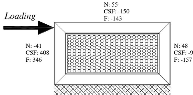
Figure 6 Displacement of experimental steel frame in middle of beam & column (Micro Strain) at 540<sup>th</sup> second of cyclic loading in samples N, CSF & F
