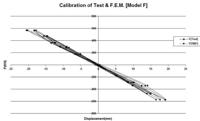
Figure 4 Comparison of experimental & F.E.M. results [F]
