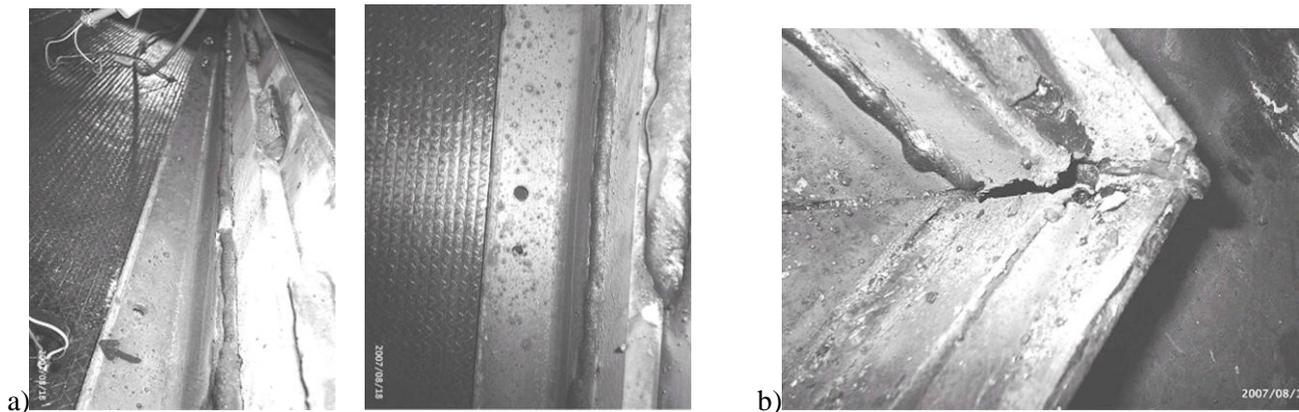
Figure 3 Demolition of connection in specimens a) FRP composite shear wall[CSF] b) Flexural Frame [F]
