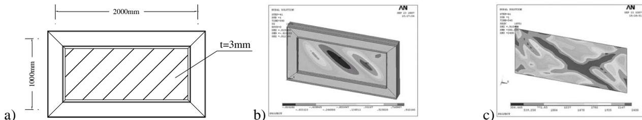
Figure 1 a) Dimension of Panel b) off-plane displacement c) Von-Misses in-plane stress of steel plate shear wall at 540<sup>th</sup> second
