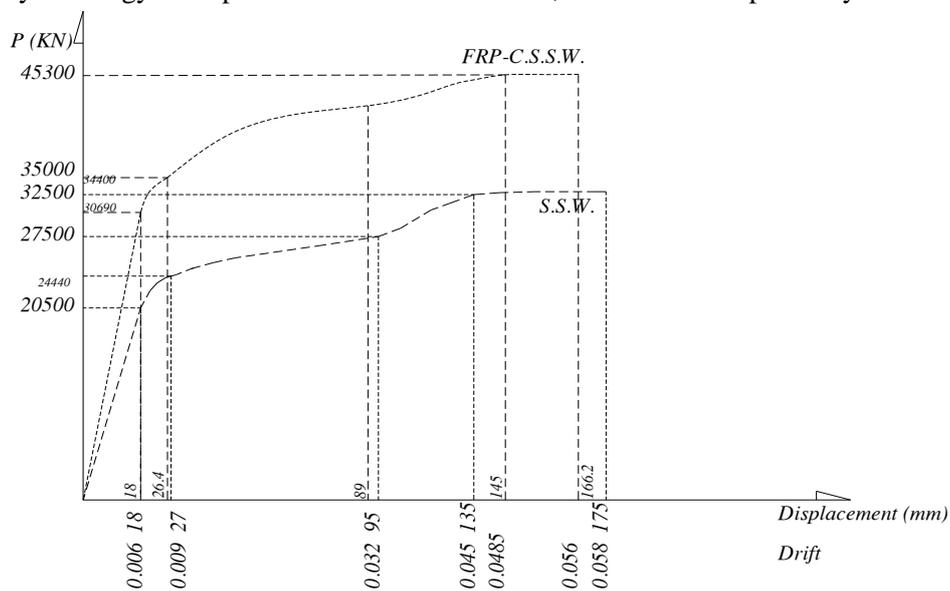
Figure 7 Numerical load-displacement push over diagram in specimens N (SSW) and CSF (FRP-CSSW)
